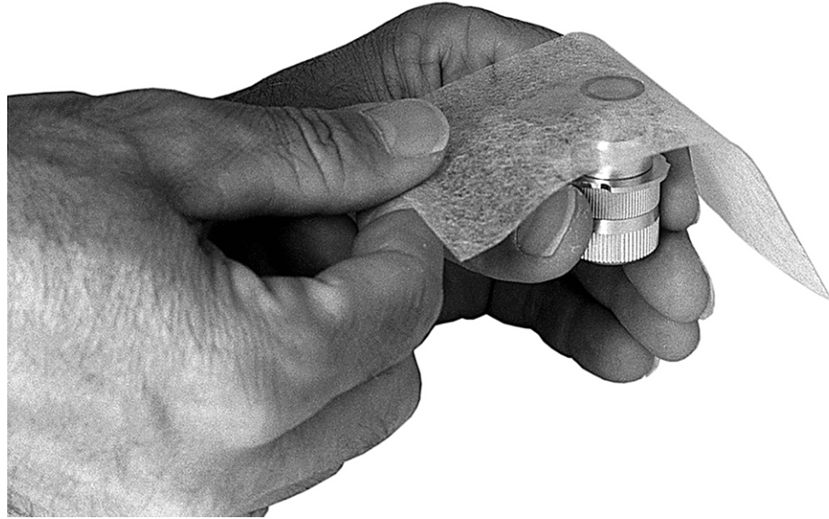
Figure 9-1: Drop and Drag Method.
