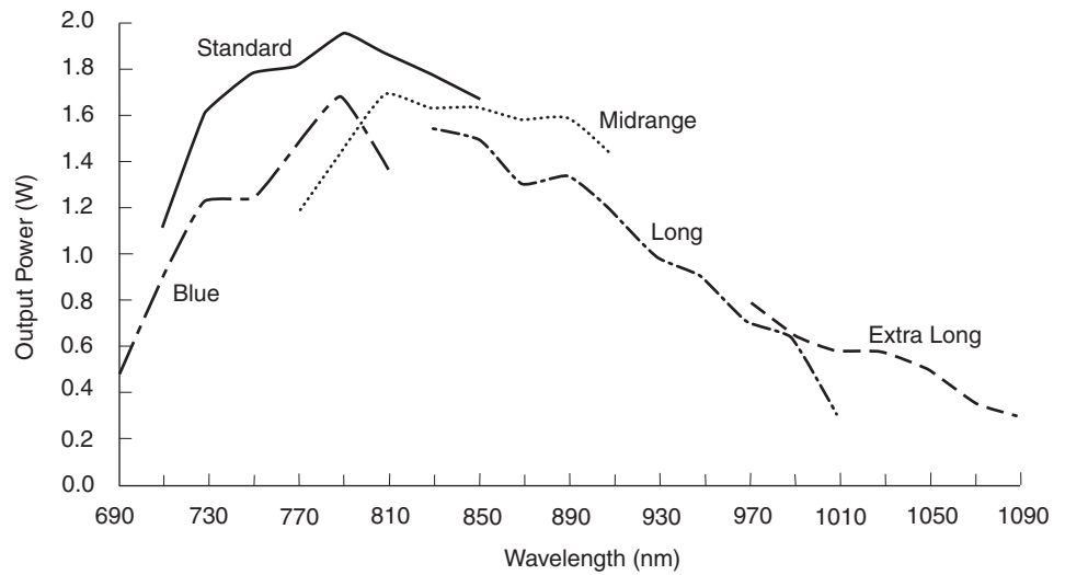
Figure 3-9: Tsunami picosecond tuning curves for the optics sets shown when pumped by a 10 W Millennia Xs diode-pumped CW laser.
