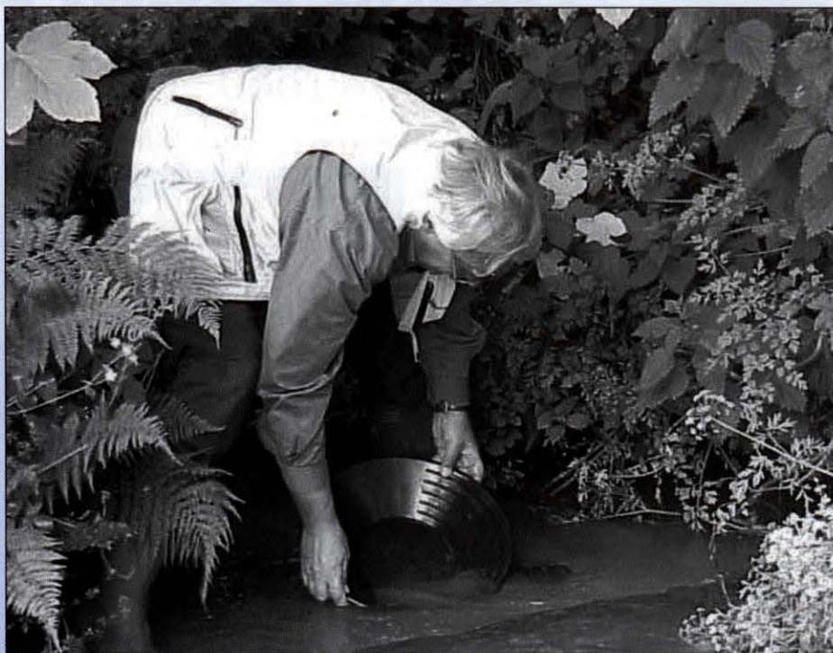
Figure 5. Dr. Simon Camm of the Camborne School of Mines, University of Exeter, illustrates how to obtain the black ilmenite sand by a classic panning procedure. The ancient Victorian miners used this same procedure for gold in this region. The ilmenite, being magnetic, can be lifted easily from the grit at the bottom of the pan. 5
