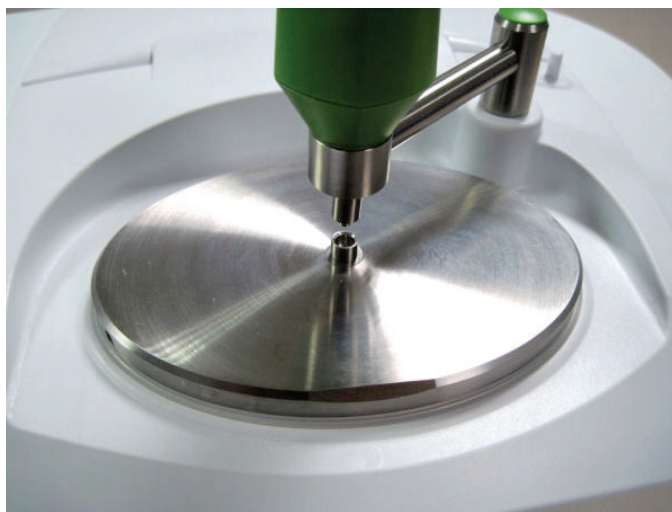
Figure 10 Using the pressure arm with a medium shoe to position the volatiles cup
