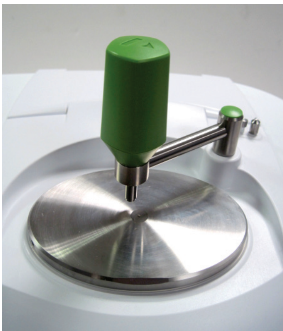
Figure 8 Moving the pressure arm into its operating position (large shoe)
