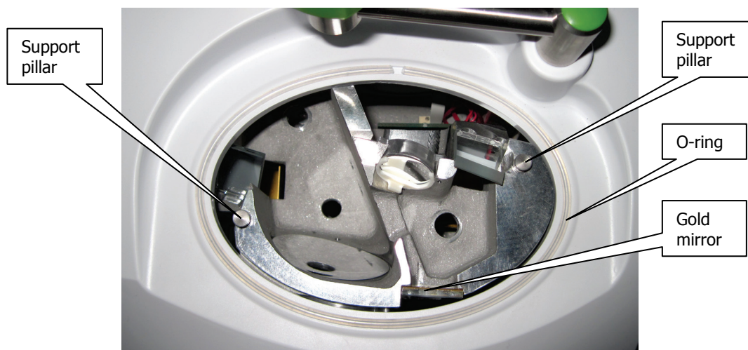
Figure 14 UATR with top-plate removed
