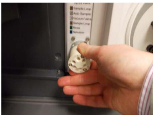
**Figure A-23.** Checking the valve seat
