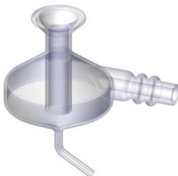
**Figure 3-5.** Baffled cyclonic spray chamber
