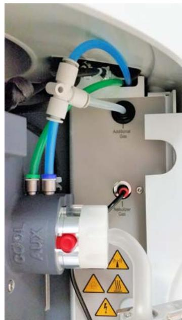
**Figure A-28.** Additional gas accessory aux gas connections
