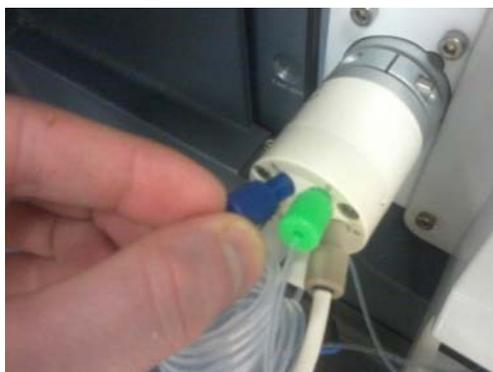
**Figure A-26.** Reconnecting the tubing
