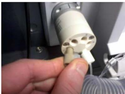
**Figure A-20.** Removing the tube connectors
