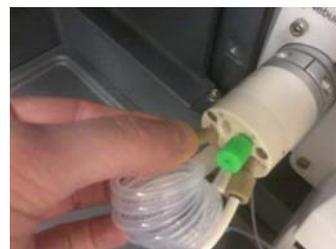
10. Screw the fitted nebulizer tube into port 6.
