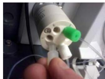
9. Attach the sample loop into ports 1 and 4 of the valve head (this is the same as the loop provided in the Field Service Test Kit).
