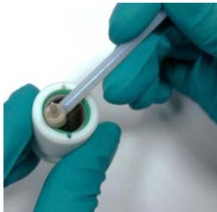
**Figure 8-5.** Inserting green O-ring
