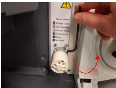
**Figure A-24.** Tightening the locking collar
