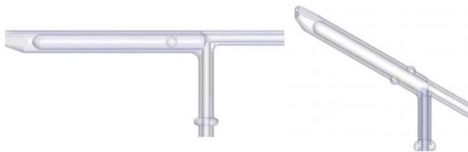
**Figure 3-6.** V-groove nebulizer for heavy organic sample analysis
