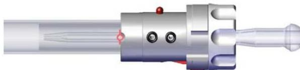
**Figure 6-19.** Torch assembly - center tube to torch mount
