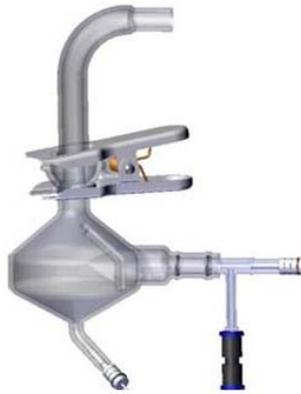
**Figure 6-12.** Spray chamber/adaptor assembly
