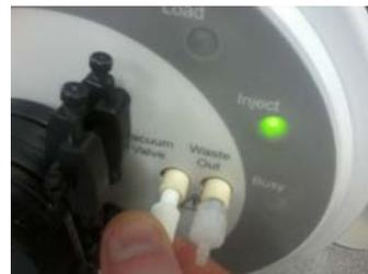
7. Attach the vacuum pump waste tubing to the waste out connector of the iCAP 7000 Plus Series ICP-OES.
