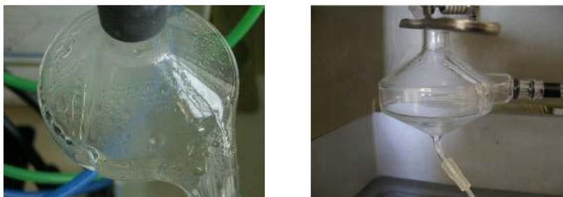
**Figure 8-1.** Spray chamber: dirty (left) - clean (right)
