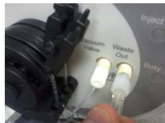
8. Screw the autosampler probe valve fitting into port 2 of the valve head.
