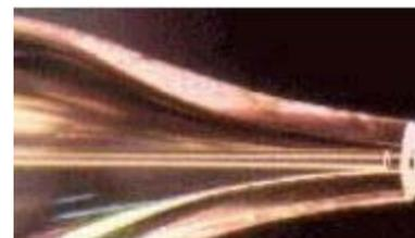
In most instances, blockage in the nebulizer is caused by either particulate matter (from the sample) or chemical deposits. It normally occurs in the nozzle where the flow passages are extremely small and constriction is greatest in the annular gas channel between the tip of the capillary and the taper of the nozzle.
