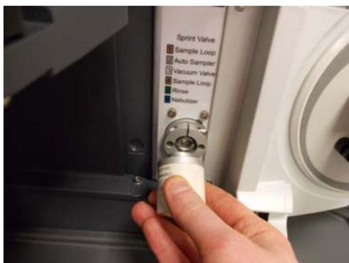
**Figure A-22.** Inserting the valve
