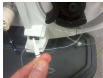
Cut a length of the supplied drain tubing so that it can reach between the pump tubing and the waste container.
