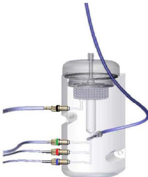
**Figure B-4.** Integrated hydride generation kit
