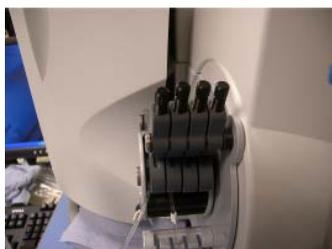
**Figure 7-2.** Peristaltic sample pump
