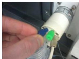
11. Attach the other end on the nebulizer line and the nebulizer gas fitting onto the nebulizer.
