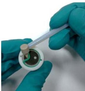
**Figure 8-4.** Removing green O-ring
