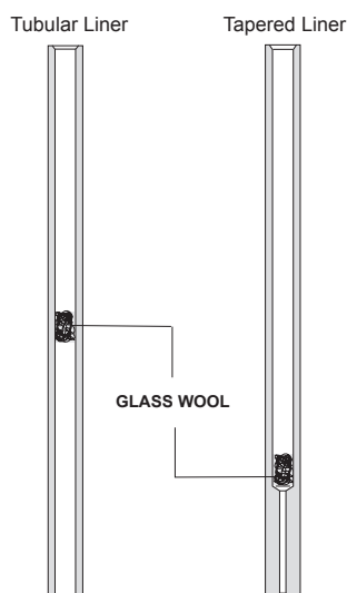
Figure 50. Packing a SSL Liner
