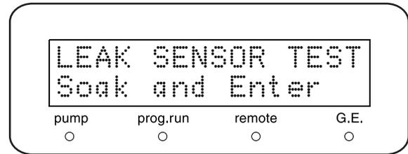
**2** Wait about 10 seconds. Then, press **enter**. If the sensor detects a leakage, [GOOD] will be shown. If not, [NO GOOD] will be shown.
