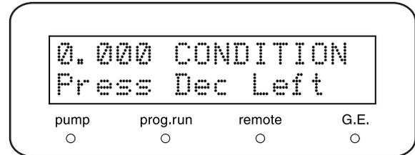
If the pressure has been at least 10% higher than the level shown 5 minutes ago, [Press Increase] is displayed.
