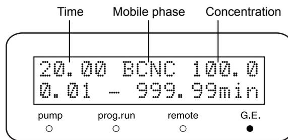
As an example of creating a high-pressure gradient program, changing the concentration of mobile phase B is shown at right. (The initial value is 0.0%.)
