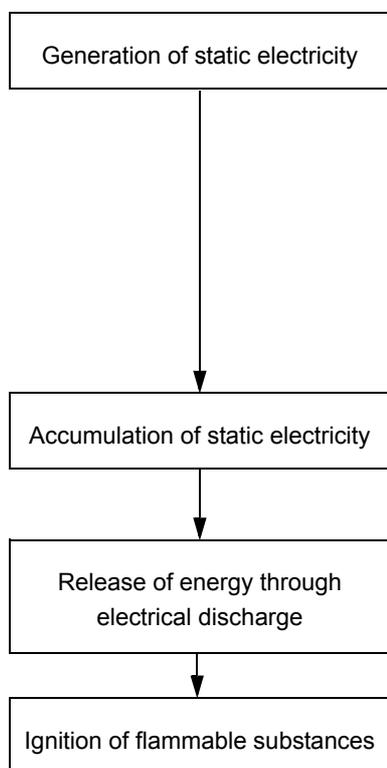
When liquid is passed through thin tubing at high flow rates, as in liquid chromatograph, the electrostatic charges of the flowing matter generate static electricity.
