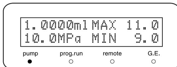
12 Change the flow rate to [1.5mL/min], and observe the pressure. When the actual pressure exceeds the [P.MAX] value set by step 11, [ERROR P-MAX] should appear.
