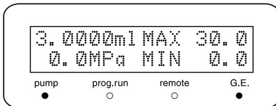
**6** Set the parameters of the control device as follows and pump until the baseline stabilizes.
