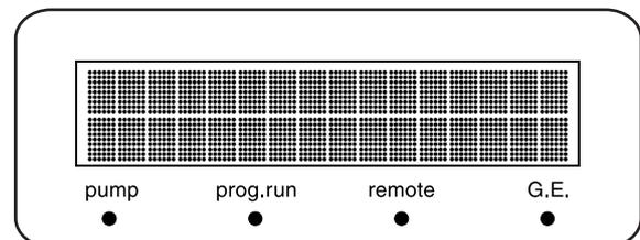
**CHECK CRITERIA : All the dots and LEDs on the screen illuminate.**
