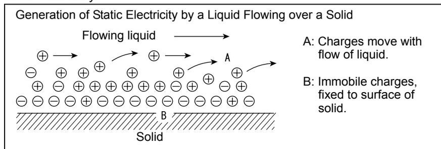
If electrostatically charged liquid is allowed to accumulate in an electrically insulated container, the charge will gradually increase, and can eventually reach several thousand volts. If this happens and an electrical conductor is brought within a certain distance of the container, electrical discharge will occur, releasing thermal energy which will ignite any flammable gas of sufficient density in the vicinity.
