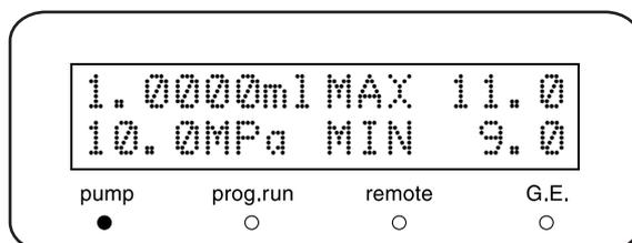
14 Reset the flow rate to [1mL/min], and press **pump** again to restart pumping.
