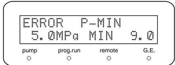
**CHECK CRITERIA : [ERROR P-MAX] and [ERROR P-MIN] appear.**
