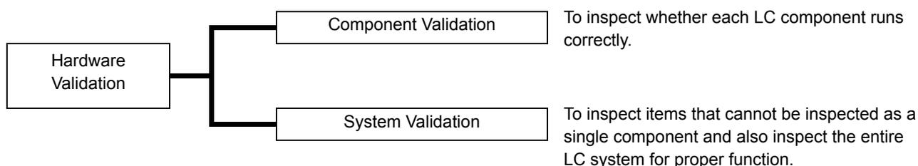
The operational protocol and criteria for this component and the HPLC system are described in this chapter to assist the user in conducting validation. Refer to each the instruction manual for each component for operational protocol of that specific component.
