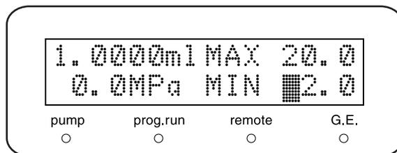
10 Press **pump** to start pumping for 1 minute.
