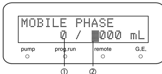
Only one type of mobile phase is shown in standard mode. However, 4 types of mobile phases (A-D) can be shown in low-pressure gradient mode.
