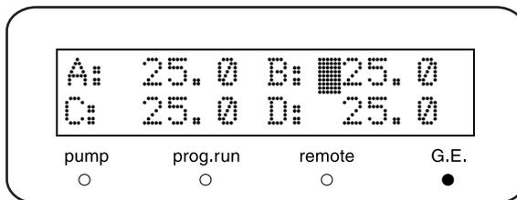
**5** Change the flow rate to 3.0mL/min, close the drain valve, and run the pumps until the baseline stabilizes.
