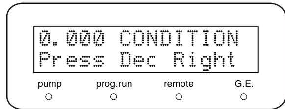
If the pressure for the left pump decreases during discharge, [Press Dec Left] is displayed.
