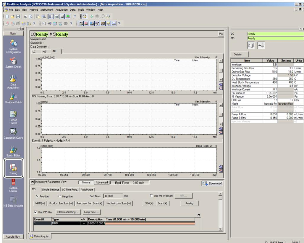
The screenshot shows the 'Realtime Analysis' software interface. The 'Tuning' window is active, displaying three chromatograms: 'LCReady MSReady', 'MS Running Time: 0.00 / 10.00 min Scan#: 0 Inten.: 0', and 'Event# 1 Polarity: + Mode: MRM'. Below the chromatograms, the 'Instrument Parameters View' is shown, including 'MS Simple Settings' and 'AutoPurge' options. The 'End Time' is set to 10.000 min. The 'Event# 1' table shows a single entry for MRM at 0.000-10.000 min.
