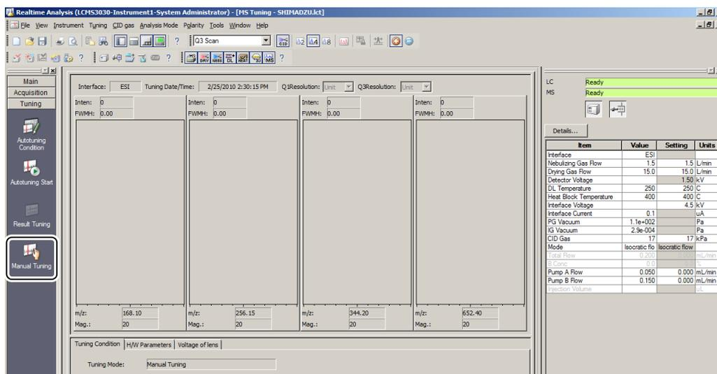
The screenshot shows the 'Realtime Analysis' software interface with the 'MS Tuning' window active. The window displays four intensity vs. m/z plots for different ions. The 'Tuning Condition' is set to 'Manual Tuning'. The 'Tuning Mode' is also set to 'Manual Tuning'.
