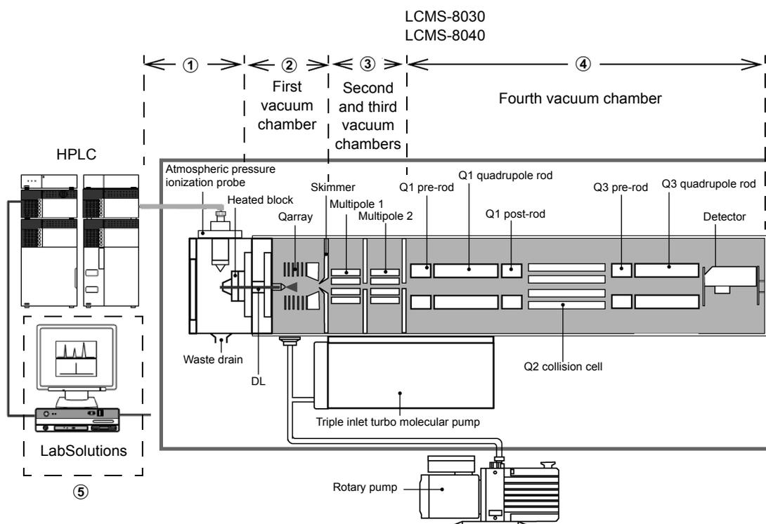
Configuration of the LCMS-8030/LCMS-8040 Unit
