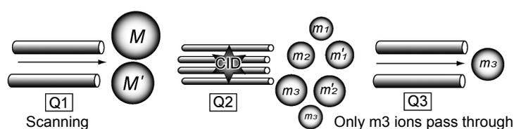
Fig. 5-4 Precursor Ion Mode Pattern Diagram
