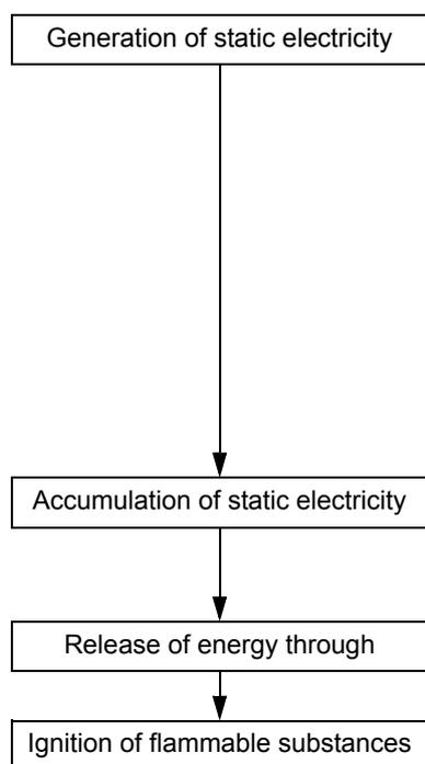
When liquid is passed through thin tubing at high flow rates, as in a liquid chromatograph, the electrostatic charges of the flowing matter generate static electricity as shown below.
