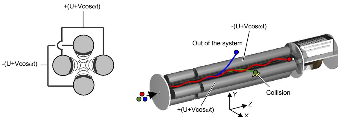
Fig. 2-21 Side View of a Quadrupole Type Mass Spectrometer
