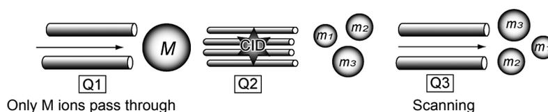
Fig. 5-5 Product Ion Mode Pattern Diagram
