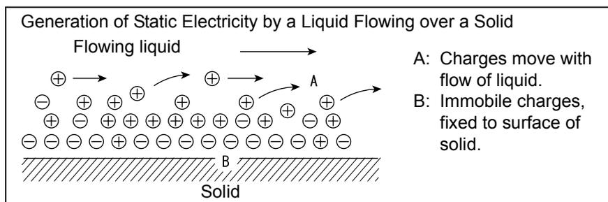
If electrostatically charged liquid is allowed to accumulate in an electrically insulated container, the charge will gradually increase, and can eventually reach several thousand volts.
