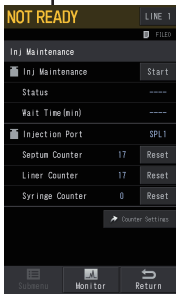
[In] Maintenance Screen
