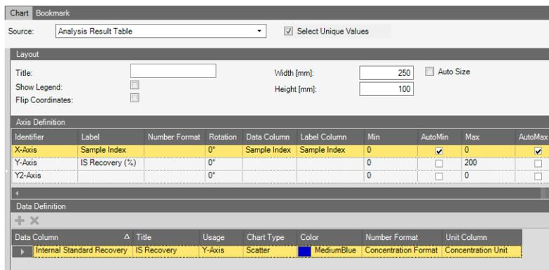
**Figure 8-59.** Example definition of an IS Recovery Report Template
