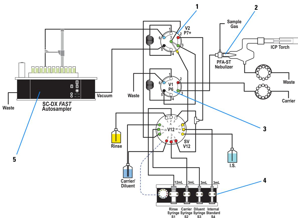
Labeled Components: 1=7-port valve (valve 2), 2=PFA nebulizer, 3=6-port valve (valve 1), 4=S400V 4 syringe pump dilution module, 5=Supporting cart
