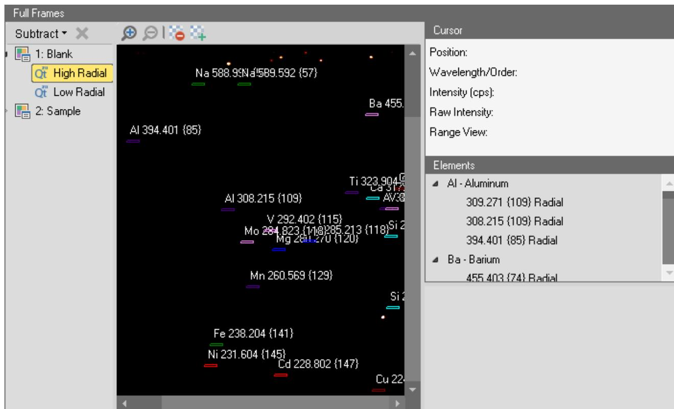
**Figure 10-52.** Full Frame results with graphical representation
