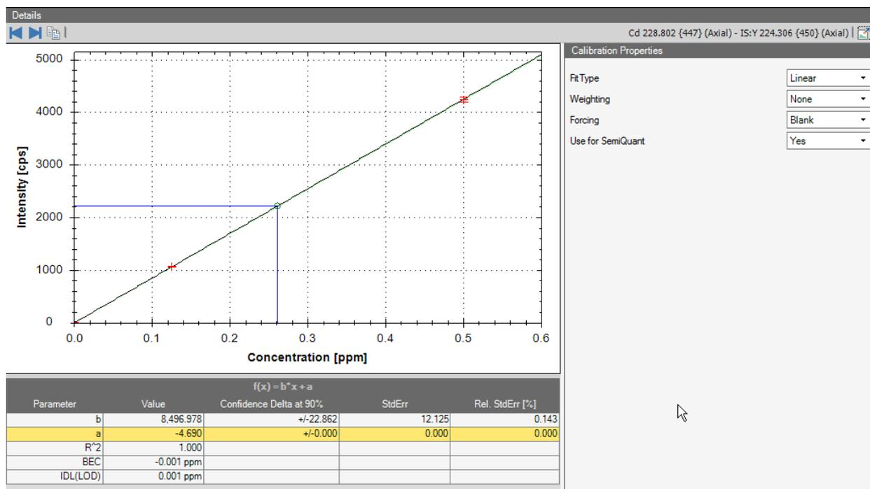
**Figure 14-23.** Calibration curve and details view of line 13 of LabBook
