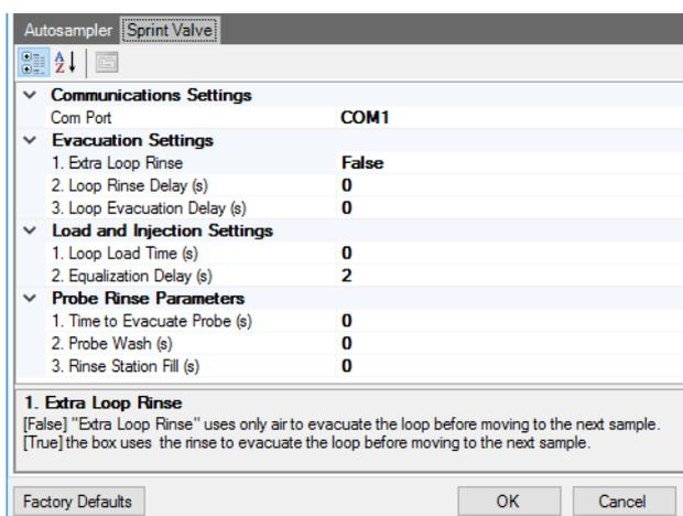
**Figure 14-45.** Typical settings for Sprint Valve
