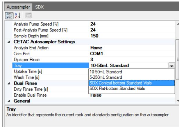
**Figure 14-43.** Tray settings for Autosampler
