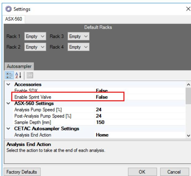
**Figure 14-44.** Settings dialog for the ASX-560 autosampler
