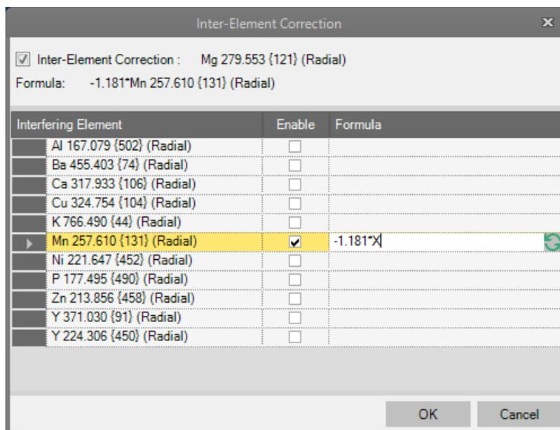
**Figure 10-46.** Inter-Element Correction dialog
