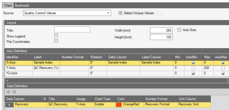
**Figure 8-62.** Example definition of a Quality Control Recovery Report Template
