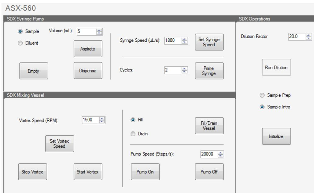
**Figure 14-47.** ASX-560 SDX tab
