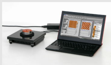
Setup. A NaioSTM, USB cable, and a PC are all you need!
