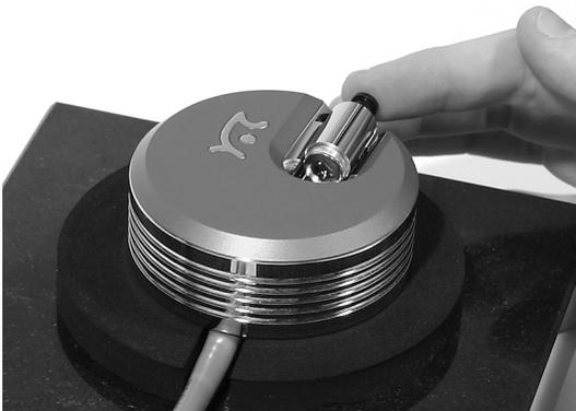
Figure 4-1: Manual coarse approach
