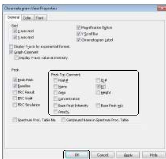
In this example, the retention time is displayed at the top of the peak.
