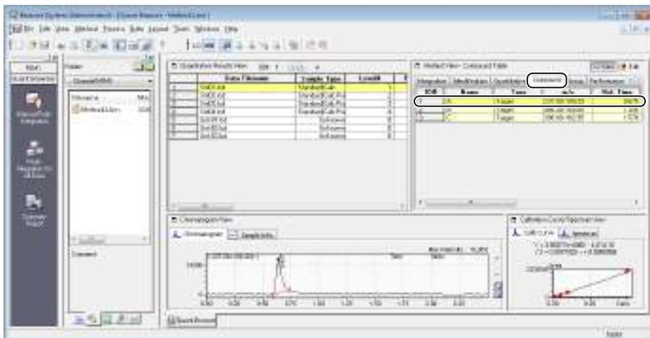
The quantitative results of the compound selected on the [Compound] tab are displayed in [Quantitative Results View], and the calibration curve is displayed in [Calibration Curve/Spectrum View].
