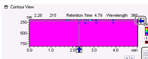
The extracted chromatogram is displayed in the [Ex] (extracted chromatogram) region in the [Chromatogram View].
