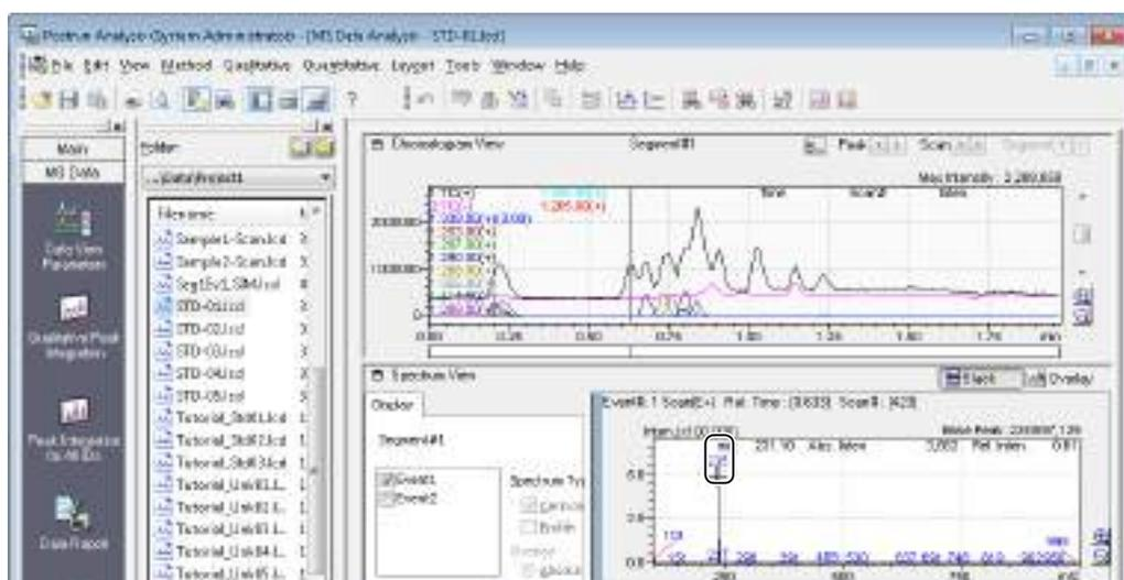
The chromatogram of that  $m/z$  is listed in the Chromatogram Table and added to the [Chromatogram View].
