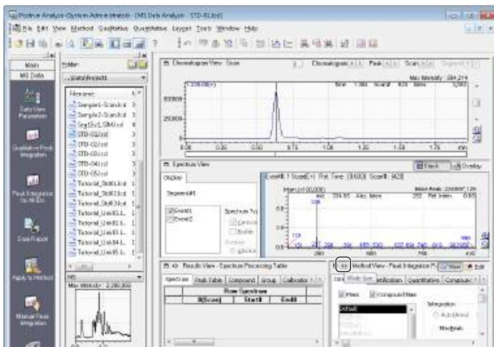
The screenshot shows the software interface with the 'Method View - Peak Integration' window open. The 'Wide Size' icon is highlighted with a red circle. The interface includes a 'Chromatogram View' showing a peak at approximately 0.75 minutes, a 'Spectrum View' showing a mass spectrum, and a 'Results View - Spectrum Processing Table'.
