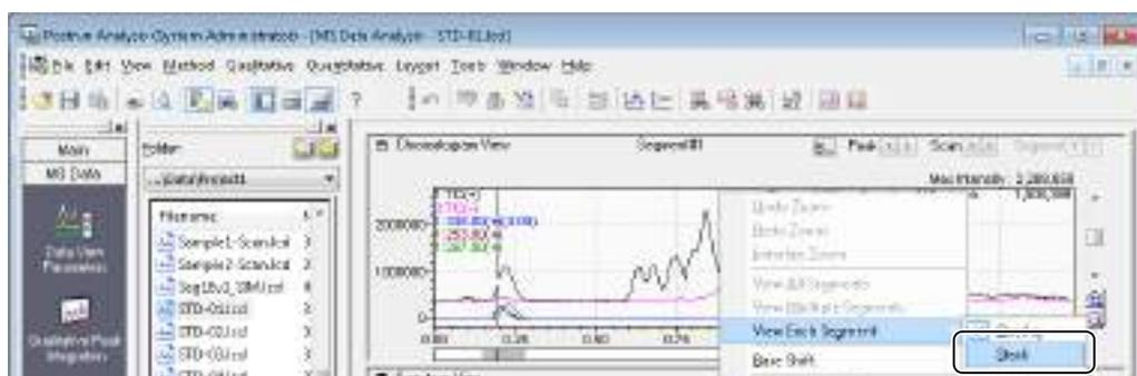
The chromatograms are displayed in a stack and the focus bar is displayed to the left of the active chromatogram.
