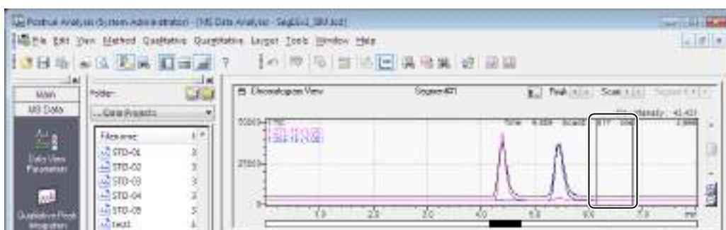
The spectrum obtained by subtracting the spectrum in the specified time range in background is displayed in [Spectrum View]. The time range averaged for subtraction is displayed in gray in [Spectrum Process Bar] at the bottom of [Chromatogram View].
