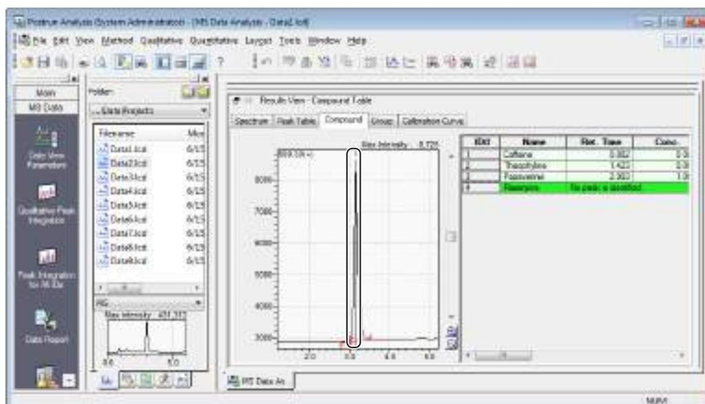
The peak is identified and the quantitative results are re-calculated and displayed in the Compound Result Table.
