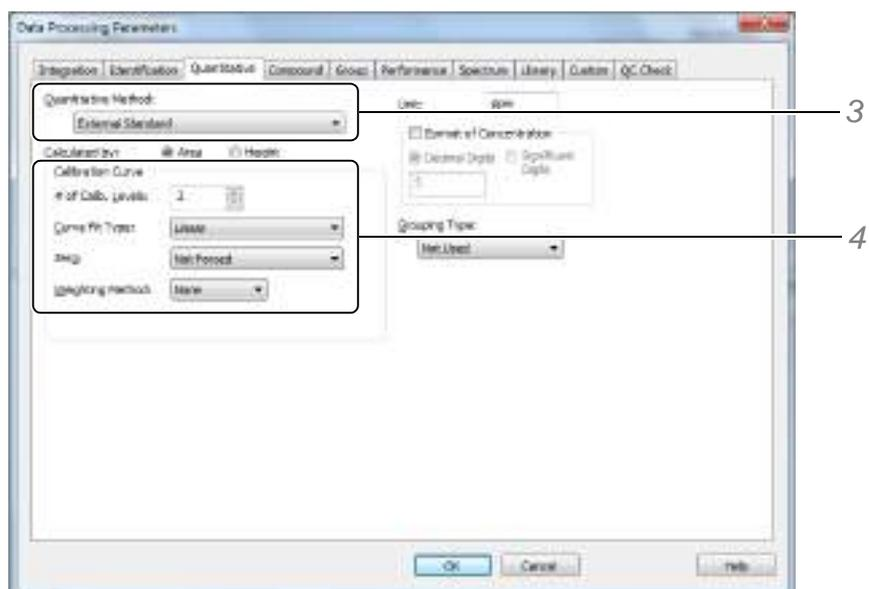
4 Set the number of levels and type of calibration curve.
