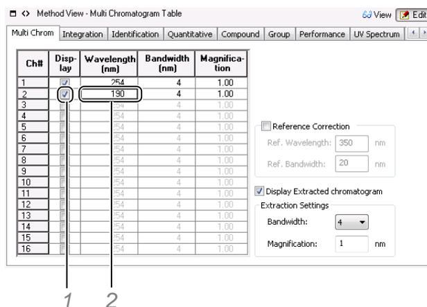
**1** Select **[Display Extracted chromatogram]** to display the chromatogram in **[Chromatogram View]**.
