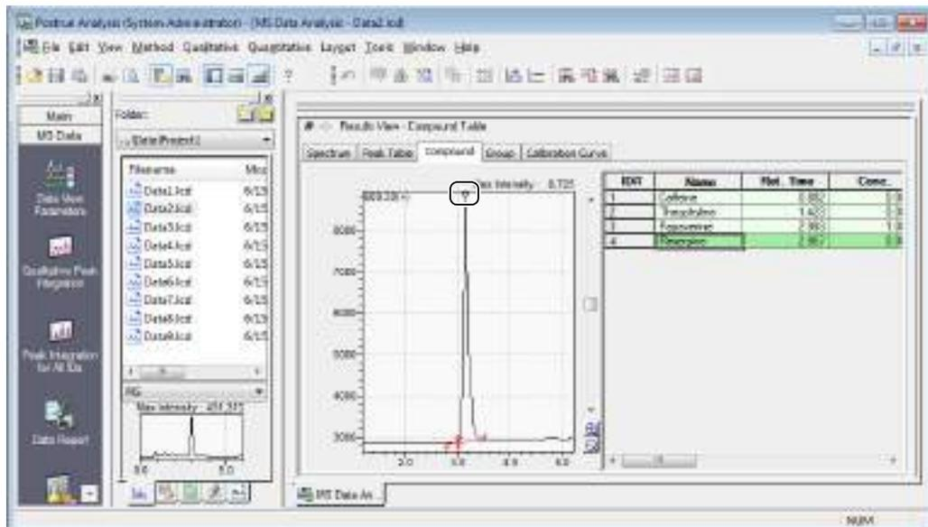
The identified peak is changed and the quantitative results are re-calculated.
