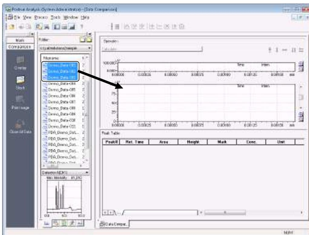
The chromatogram and Peak Table of the data files are displayed in the [Data Comparison] window.
