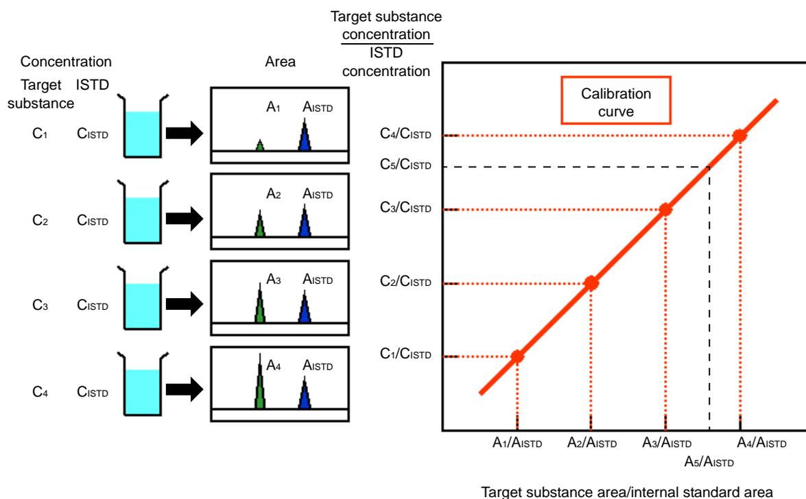
Fig.4-2 Internal Standard Method
