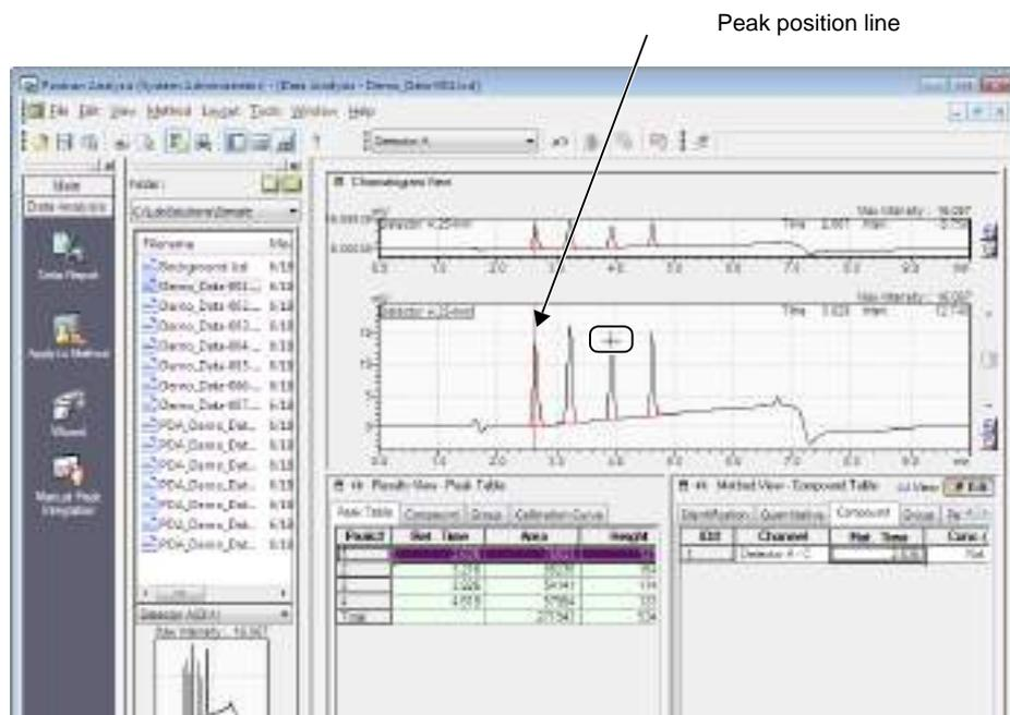
The retention time change is automatically registered to the Compound Table.
