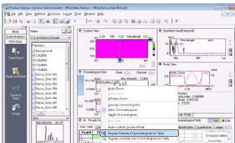
The extracted chromatogram is registered to a channel in the Multi Chromatogram Table.
