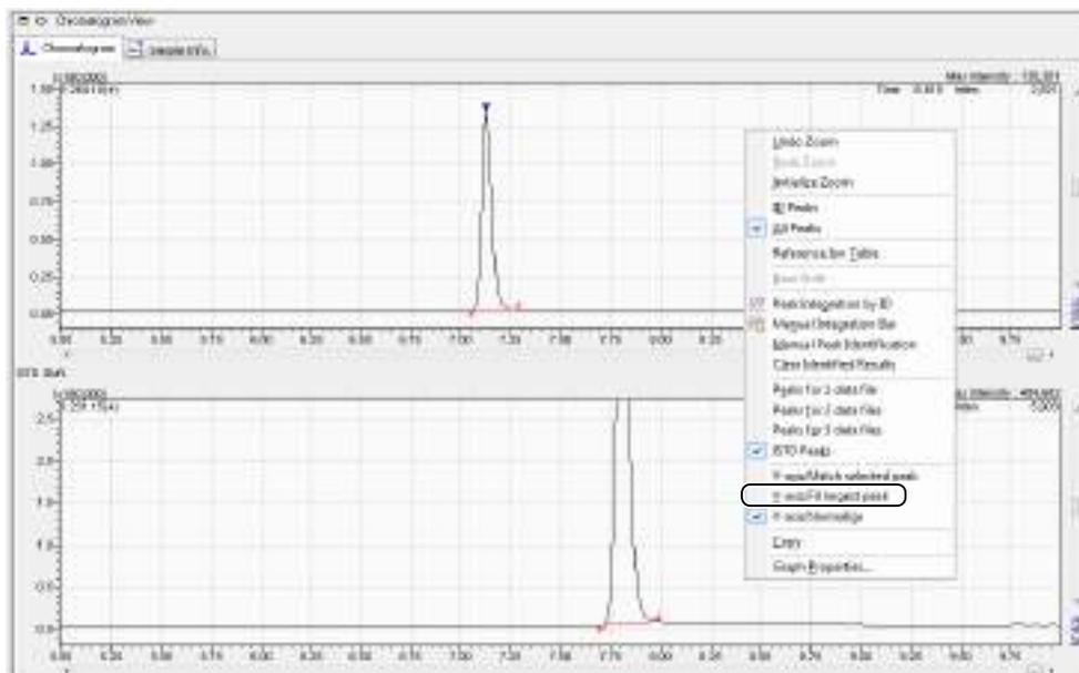
The scales of the Y axes in all the graphs are adjusted to the largest peak intensity in the displayed graphs.
