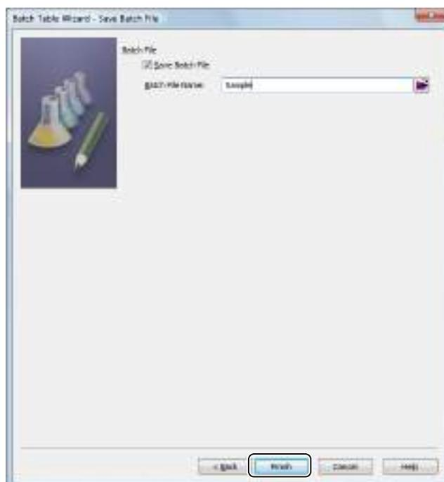
This completes Batch Table setup using the Batch Table Wizard. The batch file is created using the specified file name. This Batch Table is displayed in the Batch Table sub-window. Check the contents of the Batch Table.
