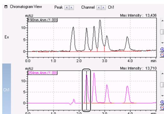
If the peak is detected, the purity of the selected peak is calculated.
