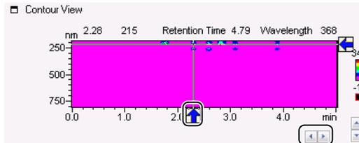
The extracted spectrum is displayed in [Spectrum View].
