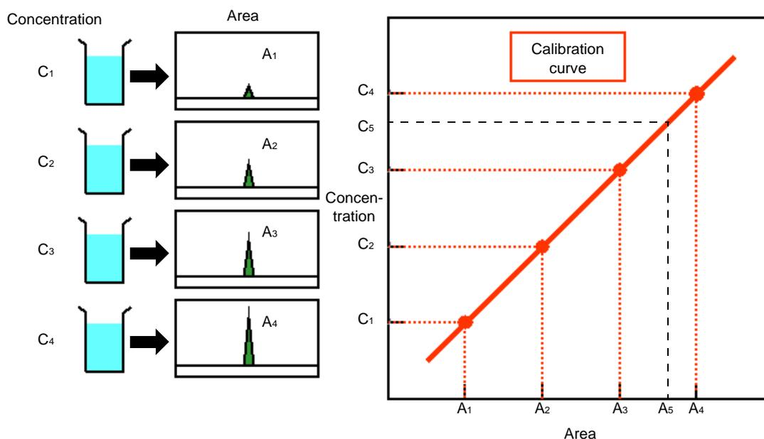
Fig.4-1 External Standard Method (Absolute Calibration Curve Method)
