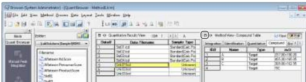
**3** Click the [Compound] tab, select the desired compound, and change [Conc. (1)]. In this example, change the [Conc. (1)] setting from “0.01” to “0.02”.
