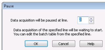
Data acquisition goes into the standby state at the selected row, and batch processing is paused.
