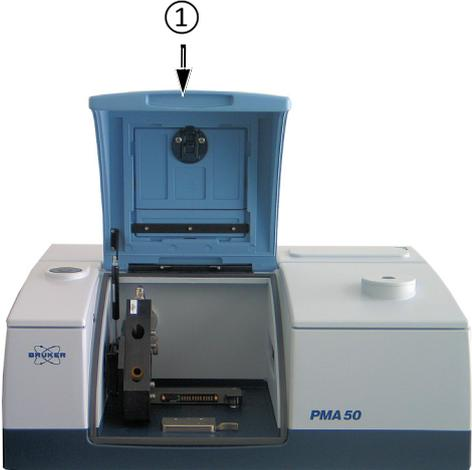
A photograph of the PMA50 instrument with its top cover open. A circled number 1 is positioned above the cover with a downward-pointing arrow, indicating the cover is turned upwards. | <p>For installing the sample holder in the sample compartment or removing it, the whole sample compartment cover ① needs to be turned upwards.</p>             |
