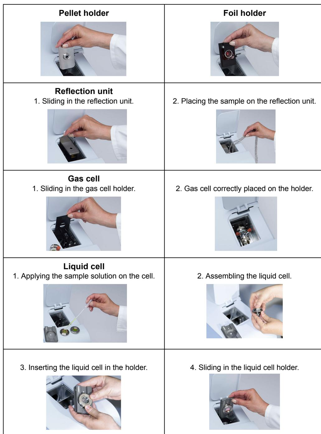
Figure 4.4: Small-sized sample compartment - Available sample accessories in use
