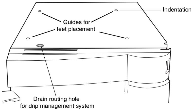
2. Place the solvent tray module atop the detector.
