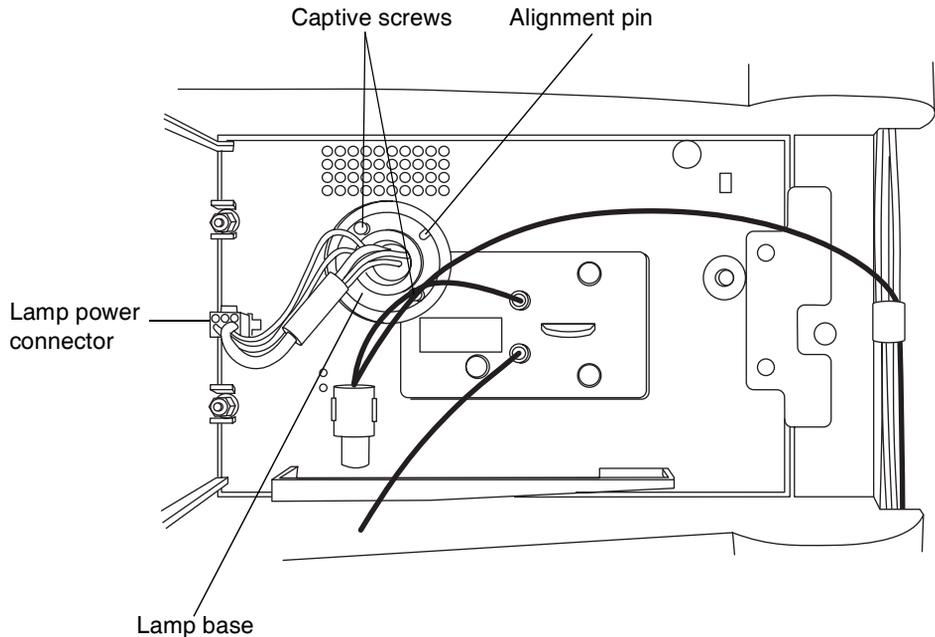
5. Loosen the two captive screws in the lamp base. Gently withdraw the lamp from the lamp housing.
