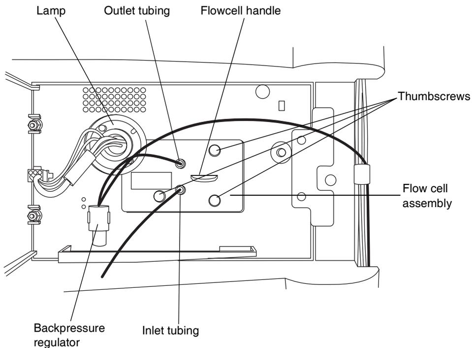
5. Remove the protective cover from the PEEK cell inlet tubing, and connect the tubing to the flow cell inlet. Confirm that the label on the tubing matches the type of detector and flow cell in your system.
