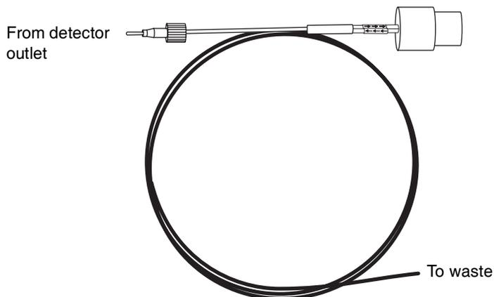
7. Route the long end of the outlet tubing from the backpressure regulator, through the channel clips along the front right side of the system, and into a suitable waste container.
