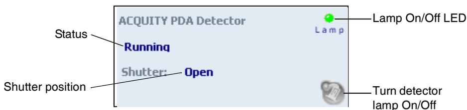
The detector control panel displays the acquisition status and shutter position. You cannot edit detector parameters while the system is processing samples.
