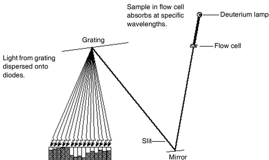
The detector measures the amount of current required to recharge each photodiode. The current is proportional to the amount of light transmitted through the flow cell over the interval specified by the diode exposure time.
