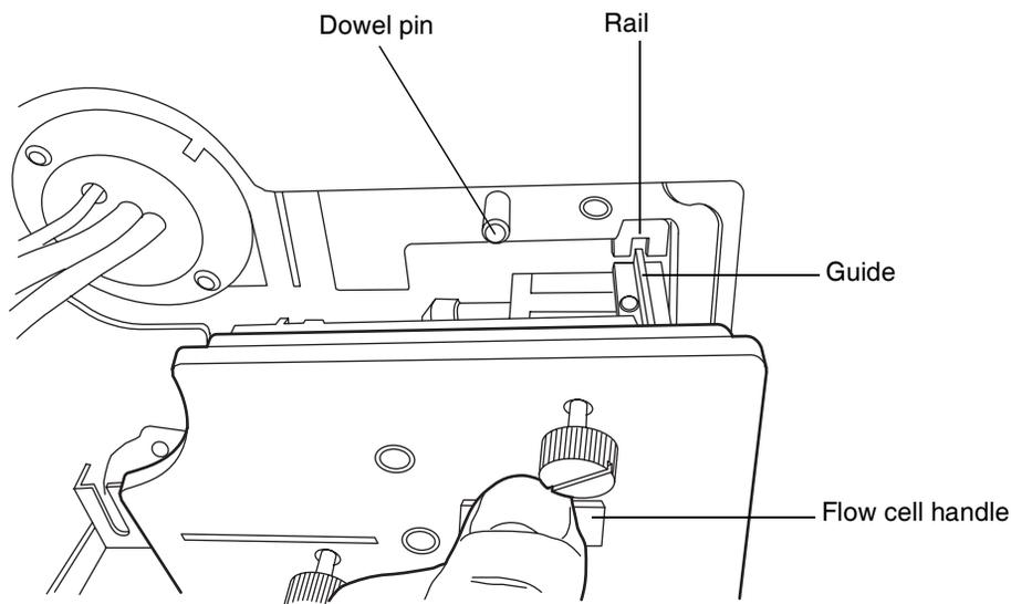
9. After the flange and rails are engaged, continue inserting the flow cell until the dowel pins on the instrument engage the corresponding holes on the cell holder.
