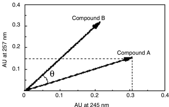
In this figure, the axes reflect the absorbance units of the two wavelengths used to calculate the absorbance ratio of the previous figure. The head of the vector for Compound A lies at the intersection of the absorbance values (for Compound A), at the two wavelengths represented by each axis. The remaining vector is similarly derived from the spectrum of Compound B.
