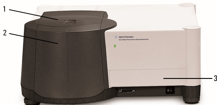
Figure 1. Cary Eclipse showing the sample compartment lid (1) and front panel (2) and Lamp Access Panel (3)
