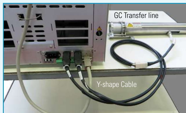
Figure 25. GC Transfer Line
