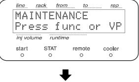
7 Press **func** until [NDL SEAL USED] appears. The needle seal's usage frequency and replacement alert value are displayed. NDL SEAL USED 0 / 40000
