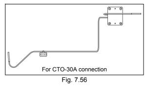
2 Straighten the wound portion of the new outlet tubing as shown in the figure.
