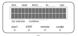
3 The memory is automatically tested, and after the memory check passes, the version number of the control program is displayed momentarily. The status indicators turns green. The screen displays the S/W version number
