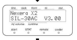
4 When the needle is in the standby state (in the injection port position), the initial screen on the right appears on the display.
