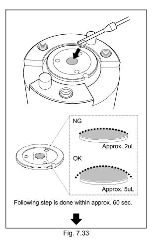
Place the stator on the high-pressure valve body within approx. 60 sec from drop of 2-propanol, and tighten three hex head bolts gently with the longer side of an Allen wrench until the bolt heads touch the stator.
