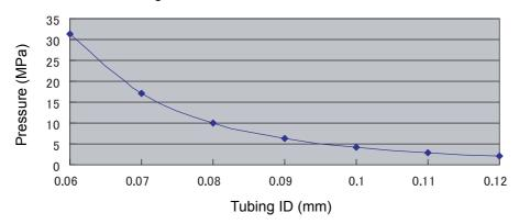
Tubing ID vs. Pressure at 1 mL/min, 20 °C
