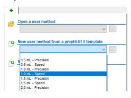
To keep the original method always unchanged, any modifications to this template are automatically saved to a user method when the **Save** button is clicked.
