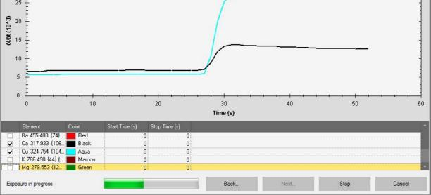
Figure 9-22. Time Study Wizard with graphical display and progress bar of exposure
