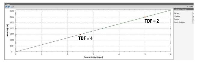
Figure 14-28. Calibration curve based on STD with 2 points of Total Dilution Factors (TDF)
