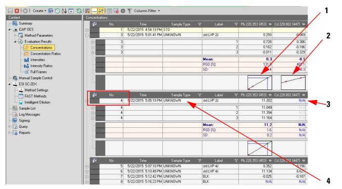
Labeled Components: 1=analyte 1 outside range, 2=analyte 2 inside range, 3=analyte 1 indicated by "N/A", 4=added new sample line
