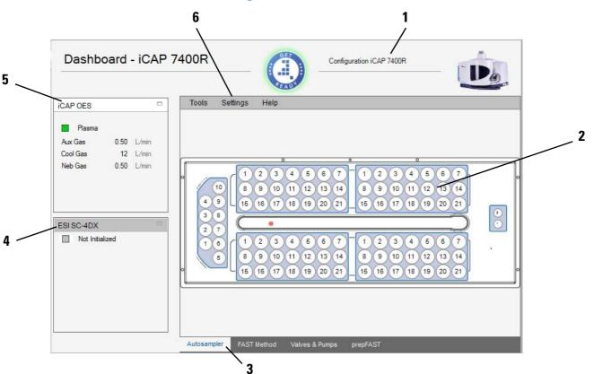
Labeled Components: 1=Configuration loaded, 2=data view region of instrument/peripheral, 3=tabs for specific settings of peripheral, 4=peripheral selector, 5=instrument selector, 6=data view menu
