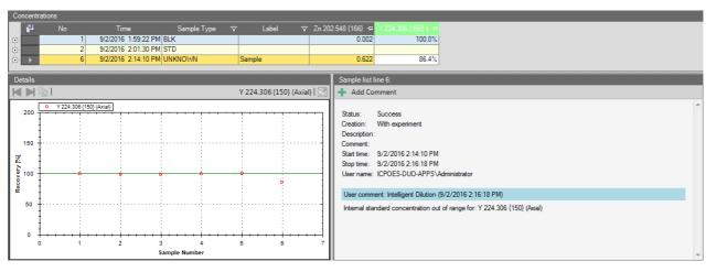
2. The measured sample has an Internal Standard Recovery of 86%.
