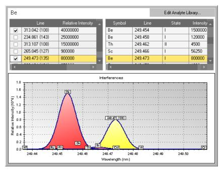
Figure 9-5. Selected interferences of an element
