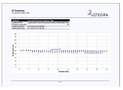
Figure 8-60. Example for an Internal Standard Recovery chart
