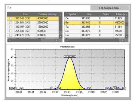
Figure 9-4. Details and interferences of an element
