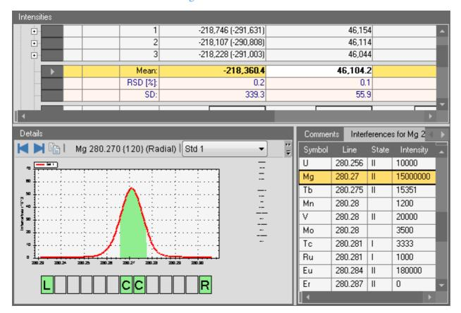
Figure 10-47. Evaluation Results: Intensities subarray plot
