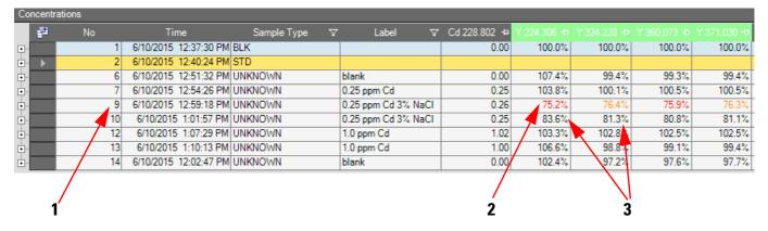
Labeled Components: 1=line number, 2=out of range values, 3=inside range values after autodilution
