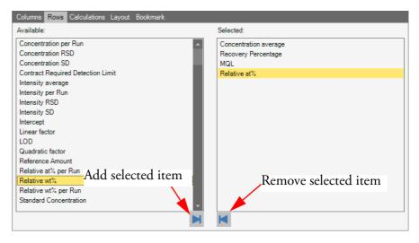
Figure 8-46. Adding or removing data types to or from Result Data Tables
