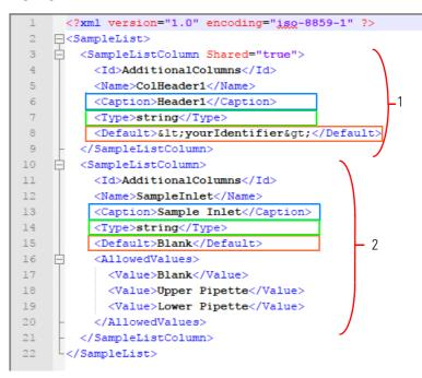
Labeled Components: 1=definition for column #1, 2=definition for column #2.
