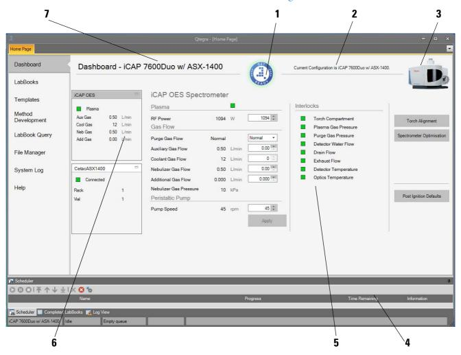
Labeled Components: 1=Get Ready button, 2=current Configuration status, 3=iCAP 7000 Plus Series ICP-OES thumbnail to change Configuration, 4=function buttons and check box for organic matrix (not shown), 5=important parameters of the iCAP 7000 Plus Series ICP-OES system, 6=instrument selector (peripheral selector), 7=current Configuration
