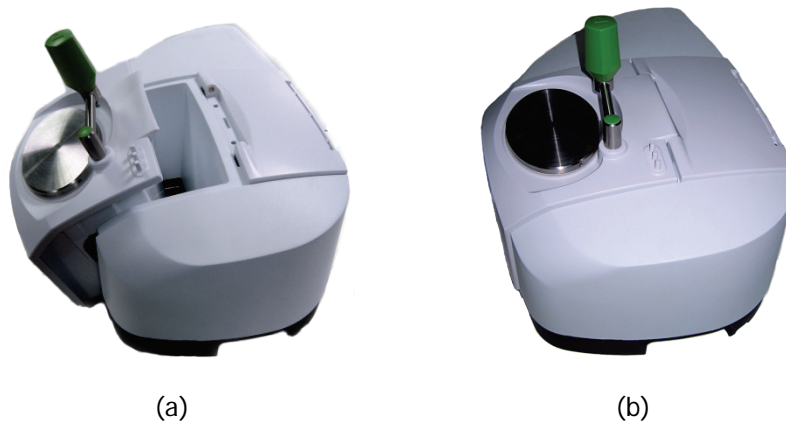
Figure 27 Installing the UATR accessory
