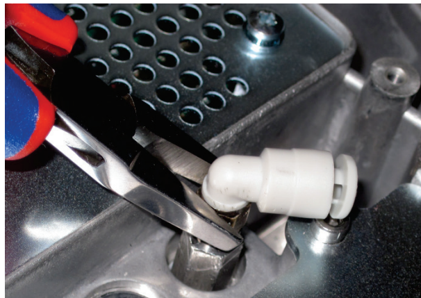
Figure 92 Tighten the purge port right-angled connector
