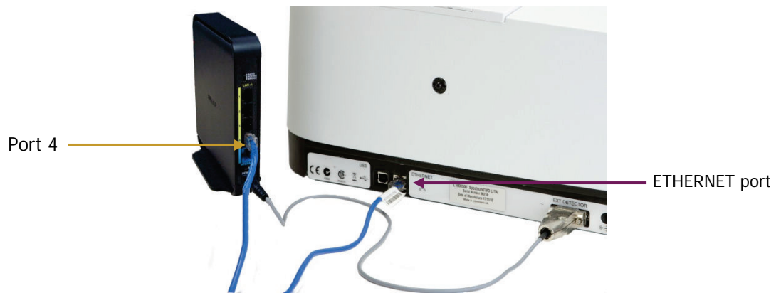
Figure 18 Ethernet cable connected to Port 4 on the wireless router and the Spectrum Two
