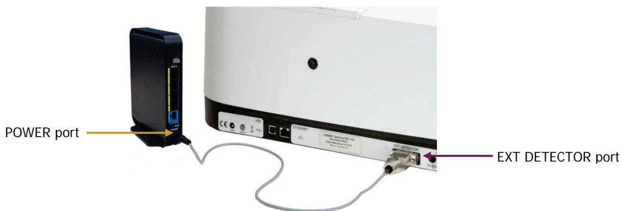
Figure 17 Wireless router connected to the EXT DETECTOR port
