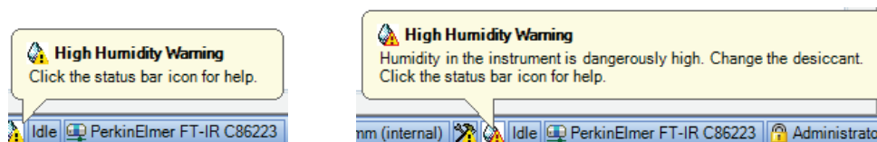
Figure 76 Humidity sensor High and Critical warning messages
