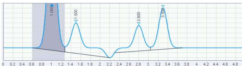
Figure 65 Integration with manual baseline between 2.3 and 3.6 min
