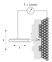
**Figure 18-1: Feedback loop.** The feedback loop maintains a constant tunneling current between the tip and the sample during motion in the X-direction by changing the Z-direction (viewed from top)
