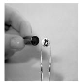
Figure 3-5: Putting the sample on the sample holder
