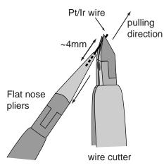
Figure 3-1: Cutting the STM tip
