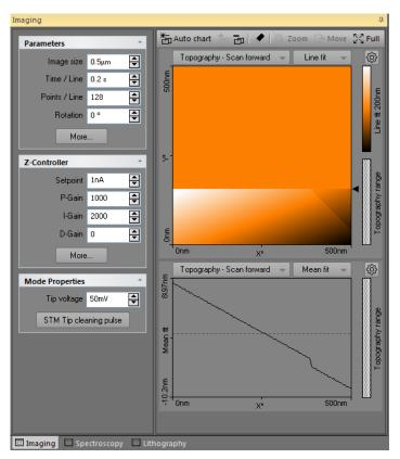
Figure 5-2: Unadjusted slope. Measurement with improperly set X\*-slope.
