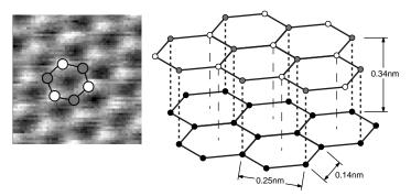
Figure 4-6: The graphite surface. (left) Measurement. (right) Lattice model.
