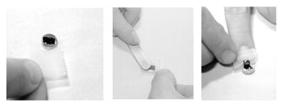
Figure 3-4: Cleaving graphite
