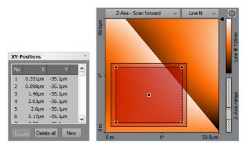
**Figure 11-2: Example of a multiple position measurement using the Grid tool.** ((Left) List of coordinates. (Right) Grid area as shown on the sample surface. Measured points are tinted bright red, measured points are tinted darker red, or according to the force curve analysis result (see ....).
