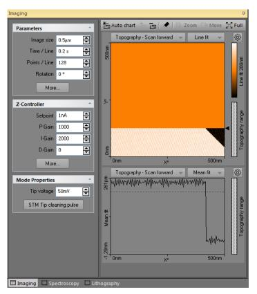
Figure 5-4: Adjusted slope. Measurement with properly set X\*-slope.
