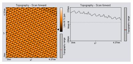
Figure 4-5: A successful graphite measurement
