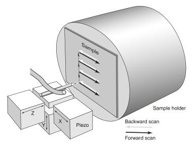
The strength of the tunneling current depends exponentially on the distance between the tip and the sample (usually referred to as Z–Distance). This extreme dependence on the Z–Distance makes it possible to measure the tip–sample movement very precisely. One of the three piezo crystals, the Z-piezo, can now be used in a feedback loop that keeps the tunneling current constant by appropriately changing the Z–Distance.
