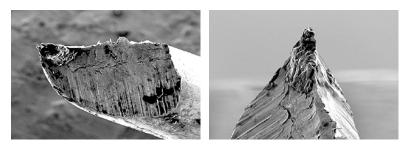
Figure 3-2: STM tip. Scanning Electron Microscope images of an STM tip
