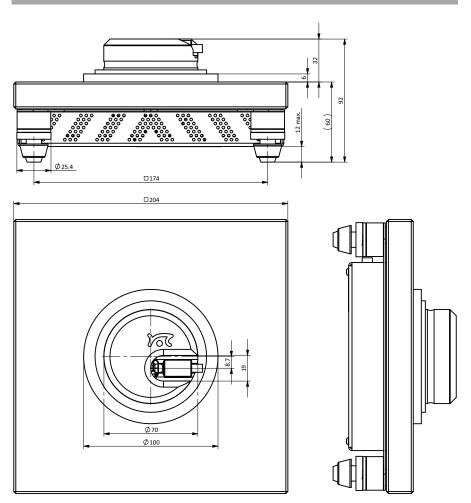
Figure 19-1: The Nanosurf NaioSTM. All dimensions in mm.
