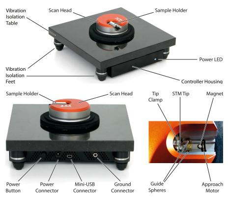
Figure 1-3: Parts of the system.
