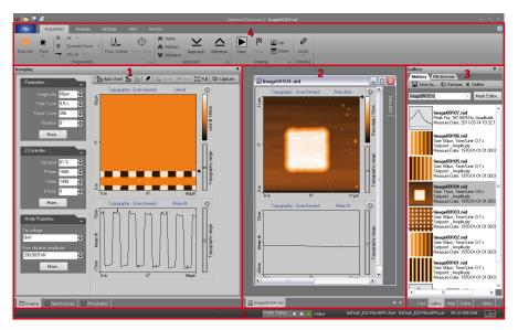
Figure 7-1: The main window in "Normal" workspace mode
