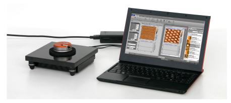
Figure 2-1: Measurement setup. Complete NaioSTM system with personal computer.
