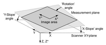
Figure 5-3: Sample and measurement orientation before slope adjustment
