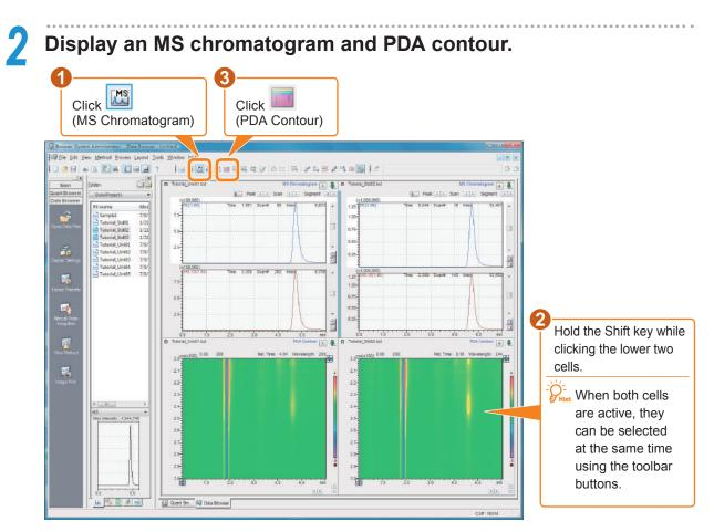
At the left side, the cell numbers of the two cells are both 1, and the same data file (Tutorial\_Unk01. lcd) is displayed in both. At the right side, the numbers of the two cells are both 4, and the same data file (Tutorial\_Std01.lcd) is displayed in both.
