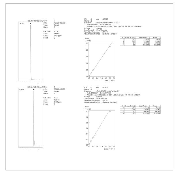
This example report for unknown sample (vial 5) shows the quantitated values for A, B and C. Also shown are the method calibration curves for A, B and C.
