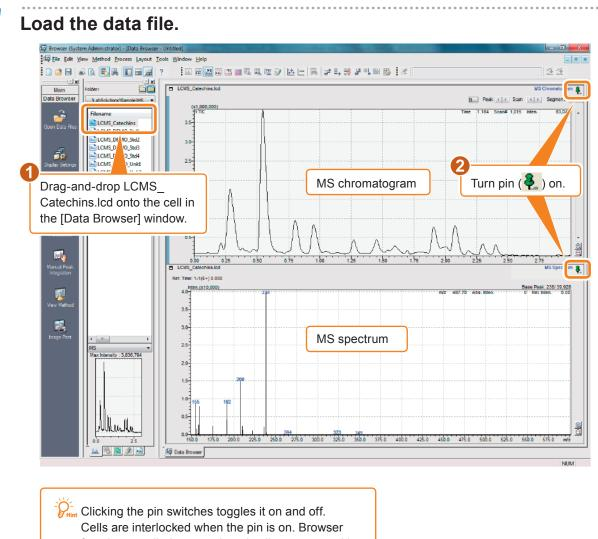
functions applied to one pinned cell are executed in all of the pinned cells.
