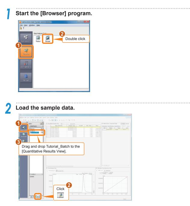
Sample data (Tutorial\_Std01.lcd to Tutorial\_Std03.lcd and Tutorial\_Unk01.lcd to Tutorial\_Unk05. lcd) registered in the batch file are opened.
