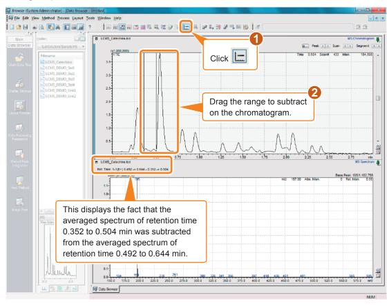
After the subtract button is selected, double-clicking on the chromatogram subtracts the spectrum at that clicked position.
