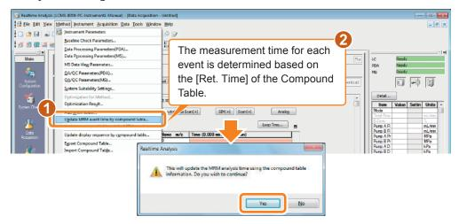
The measurement time for each event is determined based on the [Ret. Time] of the Compound Table. The start time of measurement = [Ret. Time]
