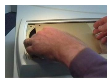
4. Undo the screw hold-down.
