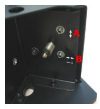
Figure 4. The vertical (A) and horizontal (B) screws are adjusted using the hex balldriver during alignment of the Fiber Optic Coupler
