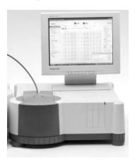
Figure 5. The Cary 50 with the Fiber Optic Coupler attached and the slotted lid in place
