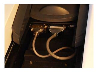
Figure 8. Connect the UMA connectors to the instrument
