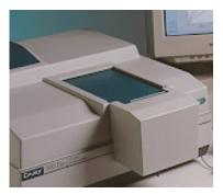
Figure 1. Extended sample compartment installed on a Cary 300
