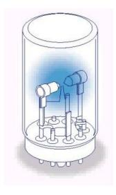
The Xenon lamp acts as a light source for the Cary 50 and 60 by emitting up to 80 flashes of light per second. Each time the lamp flashes, the Cary collects a data point.
