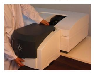
Figure 9. Install the accessory cover and slide it into place.
