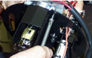
9. Remove the baffle.
