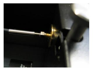
Figure 3. One end of the fiber optic probe is fitted to the port of the back of the Fiber Optic Coupler
