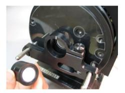
Figure 18. Inserting the powder cell into the powder cell holder
