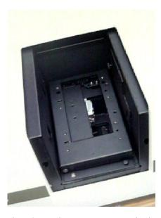
Figure 2. Sample Transport accessory in place in the sample compartment
