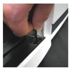
Figure 2. Loosening the screws inside the sample compartment
