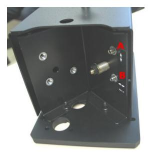
Figure 1. Fiber Optic Coupler. Note the vertical (A) and horizontal (B) adjustment ports.
