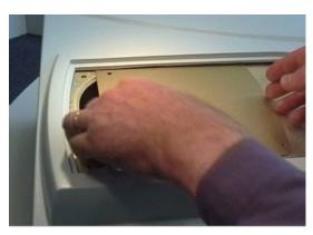
4. Undo the screw hold-down.
