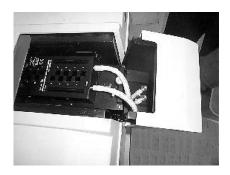
Figure 6. Attaching the Extended Sample Compartment to the instrument
