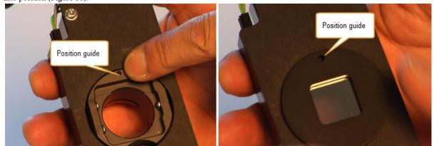
Figure 11a. Motor controller showing the location of the guide Figure 11b. Polarizing element fitted on the motor controller
