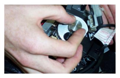
The lamp is now ready to use. No alignment is necessary when replacing the Mercury lamp.
