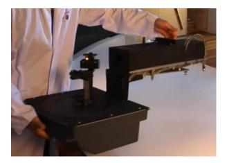
Figure 5. Lift the UMA with two hands as shown.
