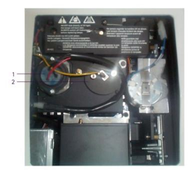
The UV lamp (1) is located next to the Visible lamp (2) in the Cary 100/300
