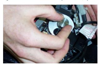
The Visible lamp should now be aligned before use.
