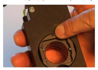
Figure 2. The Auto Polarizer motor drive unit showing the home position indicator
