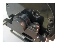
Figure 19. The powder cell fitted into the powder cell holder, note that the textured edge of the powder cell sits flush with the edge of the powder cell holder. The screw to the right of the powder cell is used to secure the powder cell.
