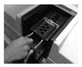
Figure 4. Sliding the top half of the 6 x 6 Multicell Holder accessory forward. The procedure is the same for the 8 x 6 Multicell Holder accessory.
