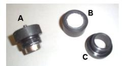
Figure 17. The powder cell. A) Lid, B) Sample cup, C) Funnel.
