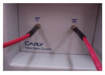
Figure 1. The end of the Reflectance probe can be fitted onto EITHER the 'Light In' or 'Light Out' channels
