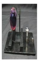
90° position for the lens (shown outside the sample compartment for clarity)
