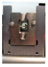
Figure 22. The double aperture base on the polarizer mount
