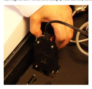
Figure 12. Auto Polarizer motor drive unit mounting slot
