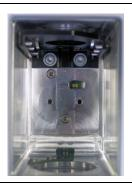
Slide bracket in the **rear position** when using the following accessories: gas cell and reflection unit
