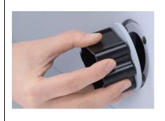
If there is not any accessory coupled to the spectrometer, the ports are closed by a blind flange. If an accessory is coupled to the spectrometer, the blind flange is substituted for a window. (Available windows are listed in section B.3.) Both the blind flange and the window are held by magnets. For removing or installing the blind flange or window from the IR beam outlet or inlet port use the special tool which is included in the delivery scope.
