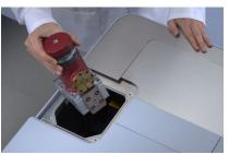
2. Take the detector straight upwards out of the dovetail guide.
