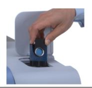
Pellet holders, magnetic holders for films, clamp holders for different kind of flat samples and liquid cells can be used.
