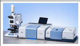
FT IR microscope of the HYPERION series coupled to the left side and a PMA50 module coupled to the right side of INVENIO R
