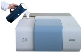
Pour slowly liquid nitrogen in the funnel. Avoid spilling the liquid on the spectrometer housing. At first the liquid nitrogen evaporates and streams out again.
