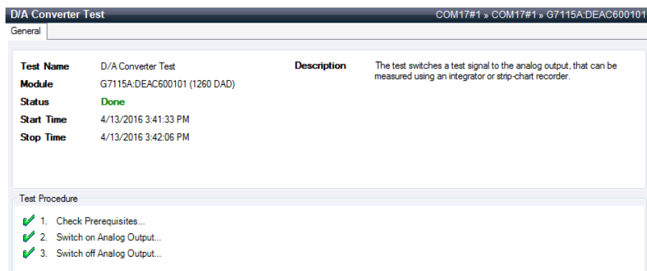
Figure 41 D/A Converter (DAC) Test – Results
