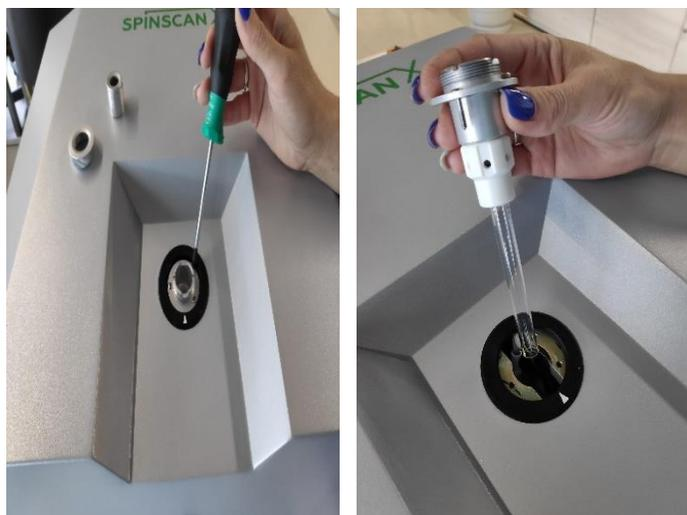
5. Detach the protective quartz tube of the resonator;
