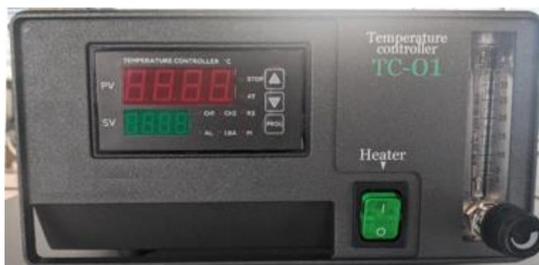
25. The Controller can be tuned either manually (on the TCS instrument panel) or using the PC software for faster and more accurate temperature control system operation. This procedure is performed when the temperature control system is first started, or when the operating modes are changed (transition from one mode to another). Autotuning is performed under the experimental conditions and at the average temperature of the experiment.
