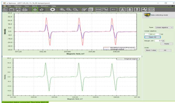
Figure 7.9 – Operation with linear algebra
