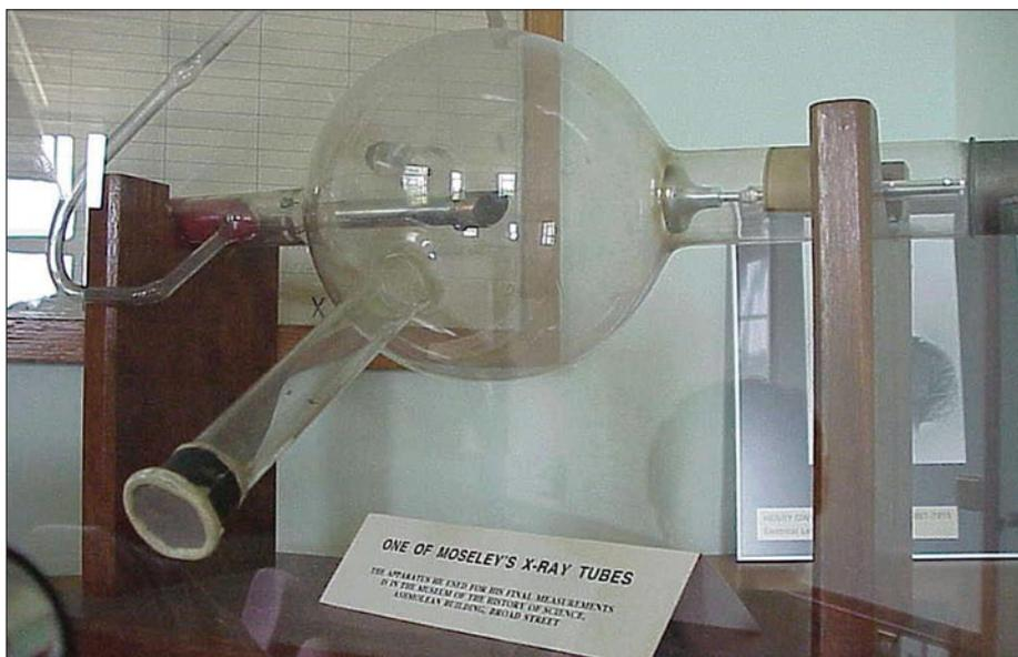
Figure 10. X-tube used by Moseley in Oxford, constructed there since the one he used at Manchester had been broken (on exhibit in the Lindemann Hall Moseley Room).
