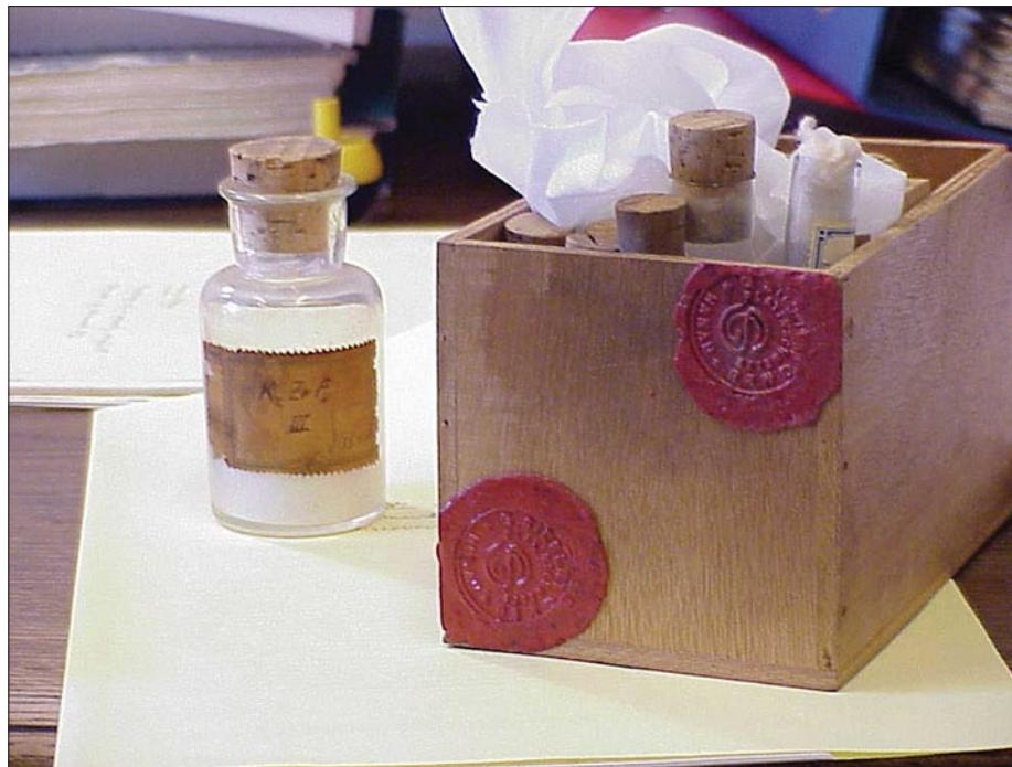
Figure 8. The "shoeshine box" full of "Hevesy's Chemical Collection," includes samples of  $K_2ZrF_6$ ,  $K_2HfF_6$ ,  $HfOCl_2$ , and other compounds prepared by Hevesy. Hevesy discovered that potassium hexafluorohafnate ( $K_2HfF_6$ ) is more soluble than potassium hexafluorozirconate ( $K_2ZrF_6$ ). Repeated recrystallizations slowly led to an enrichment of the hafnium compound in the soluble portion.
