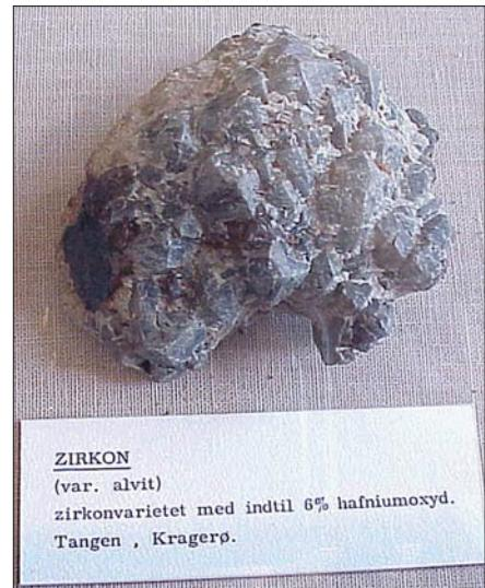
Figure 4. Hafnium-rich specimen of alvite was used by Coster and Hevesy for their studies. Gemmy crystals of zircon can be pure  $ZrSiO_4$ , but alvite is a less attractive variety which contains typically 5–10% hafnium ( $Zr/HfSiO_4$ ). This specimen containing 6% hafnium was collected at Tangen Mine, Kragerø, Norway, the source of Coster and Hevesy's minerals.
