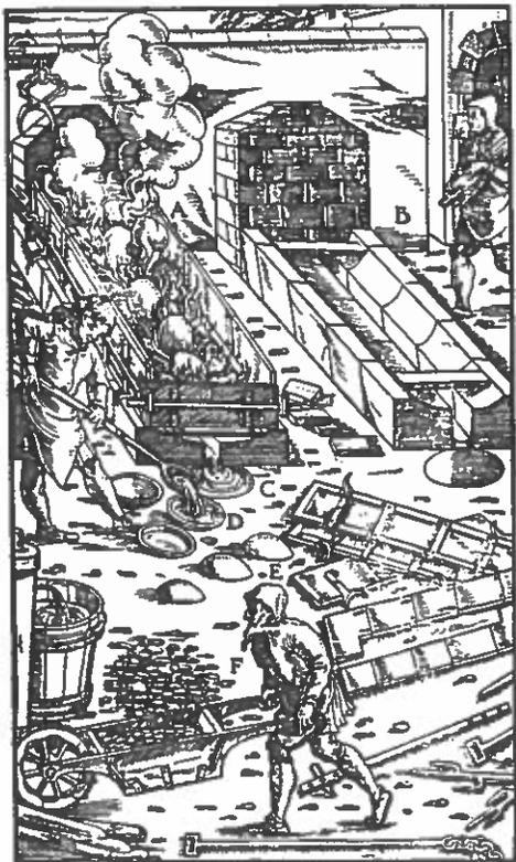
Figure 16. Smelting lead ore, from Agricola's *De Re Metallica*.
