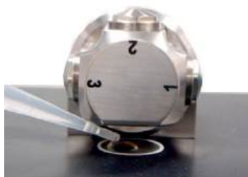
Figure 16. Placing sample on the DialPath accessory sample mounting window.
