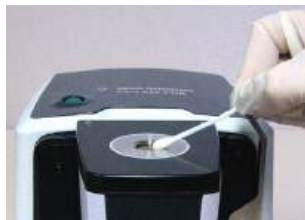
Figure 8. Cleaning the 5 bounce ZnSe ATR sampling window.
