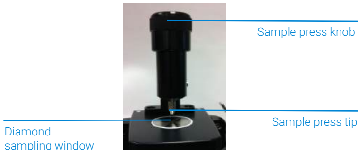
Figure 5. Diamond ATR accessory sample press in highest position.
