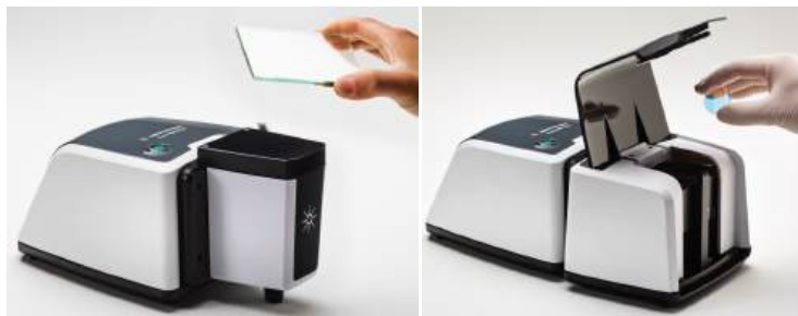
Figure 12. Sample introduction for the 10 degree and 45 degree SRA accessory.
