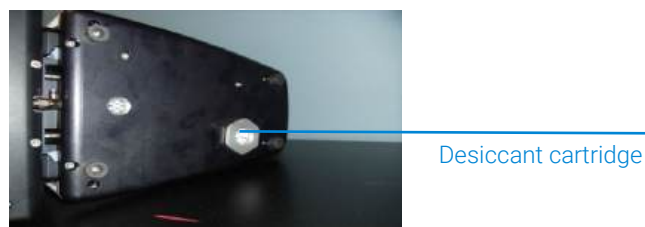
Figure 21. Desiccant cartridge location on bottom of Cary 630 FTIR.
