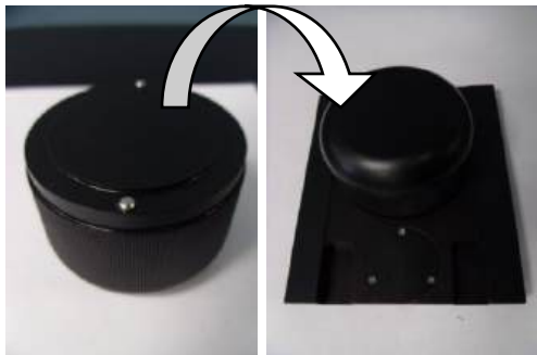
Figure 23. Window replacement tool and replacing locking ring.
