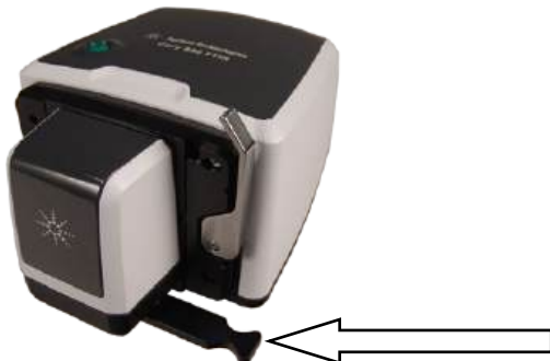
Figure 18. Diffuse Reflectance accessory attached to Cary 630 FTIR. The sample holder pushes into the slot on the lower right of the accessory.
