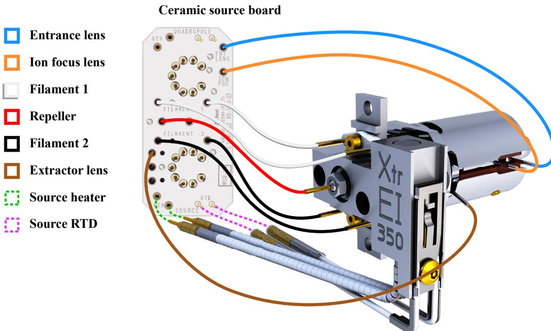
Figure 58 Wiring for the EI HydroInert Source
