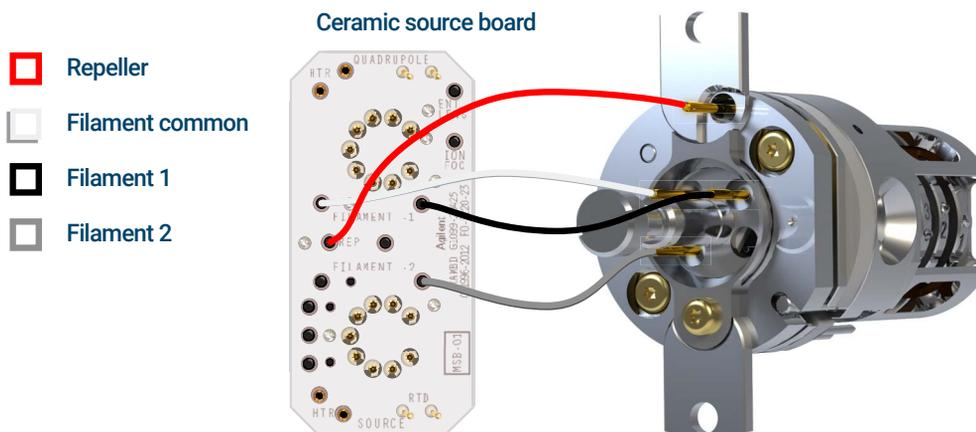
Figure 50 Wiring to be connected/disconnected during source installation or removal.
