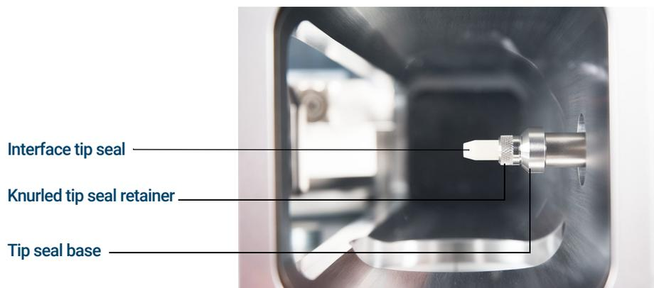
Figure 18. GC/MSD interface tip seal
