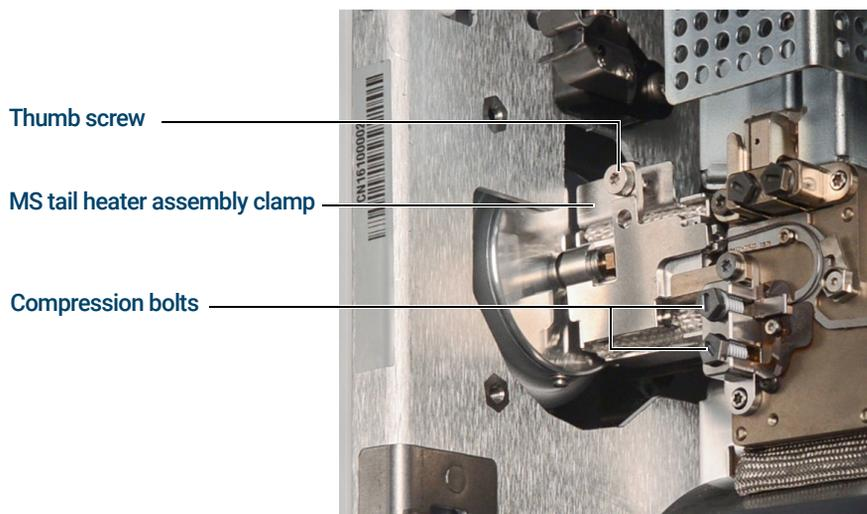
Figure 15. MS tail heater assembly clamp closed
