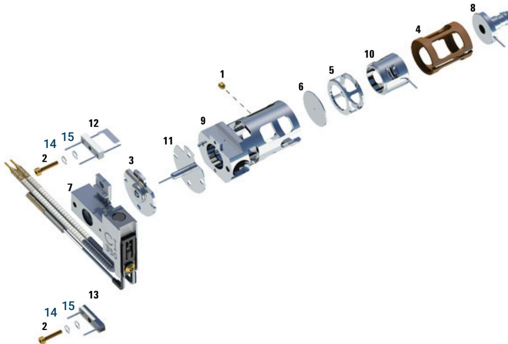
Figure 78. Assembling the CI source
