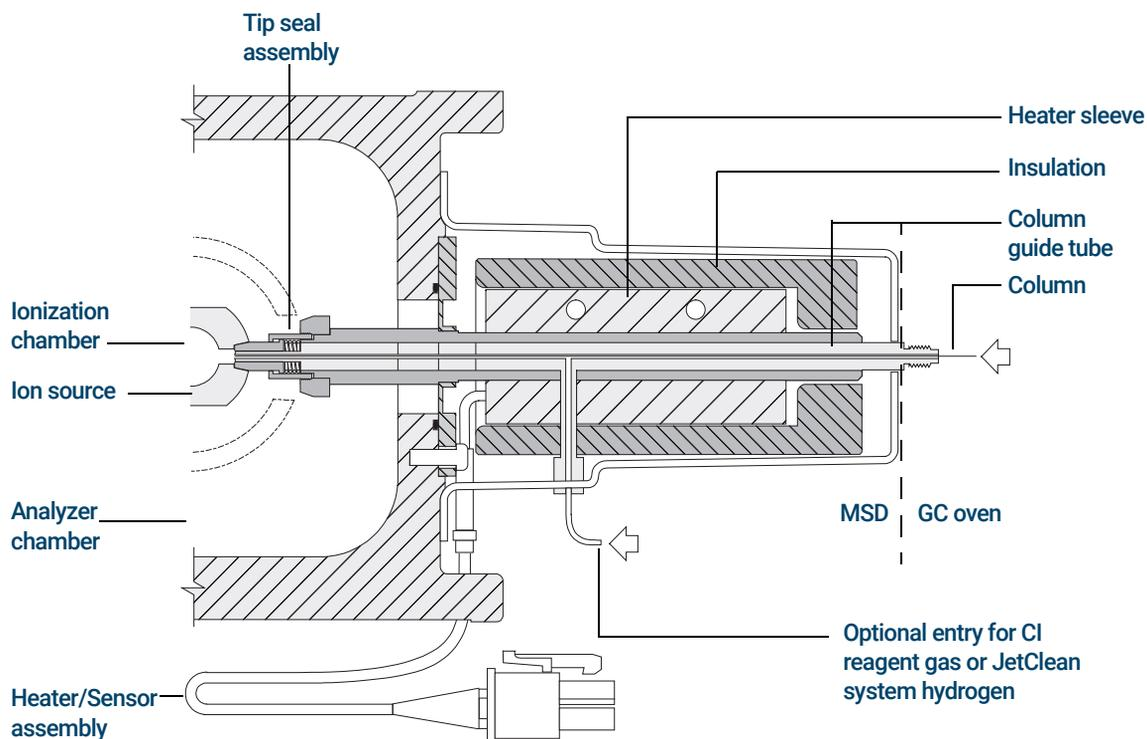
Figure 9. GC/MSD interface for an 8890 GC with EI XTR, HES, and CI sources
