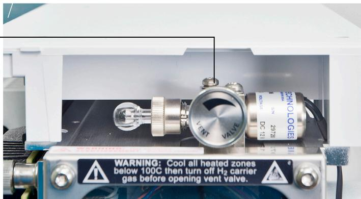
Figure 40. Vent valve knob
