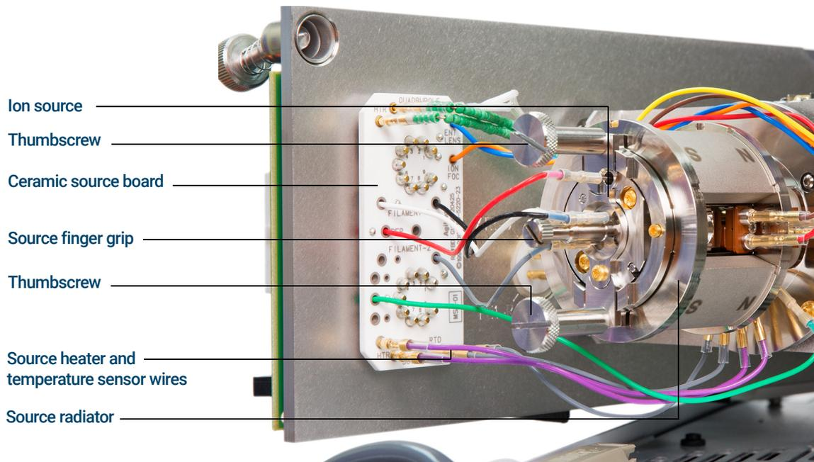
Figure 49 The analyzer chamber for the HES MSD
