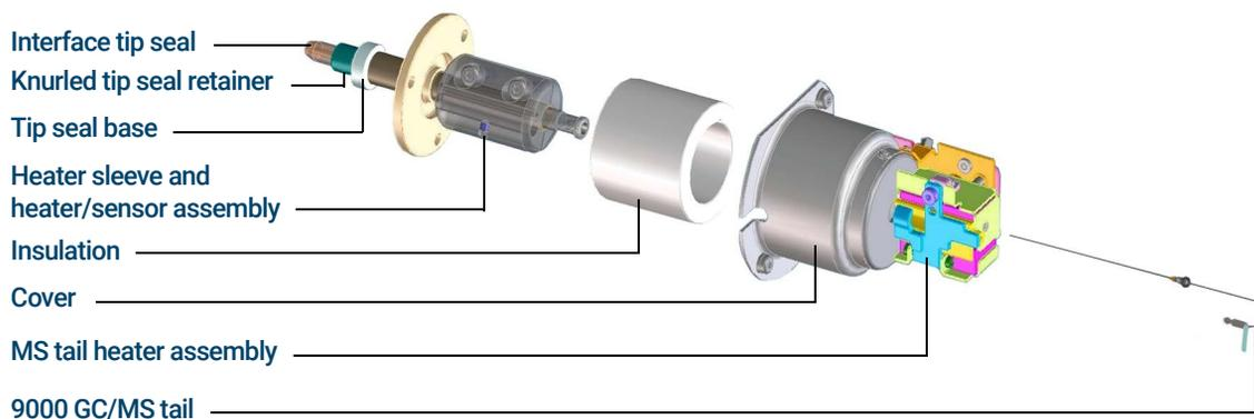
Figure 19. The GC/MSD Interface for a 9000 GC (not to scale)
