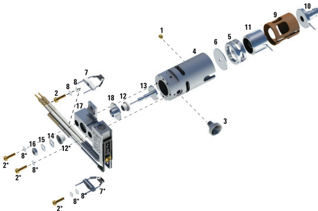
Figure 59. Disassembling the EI SS or Inert source
