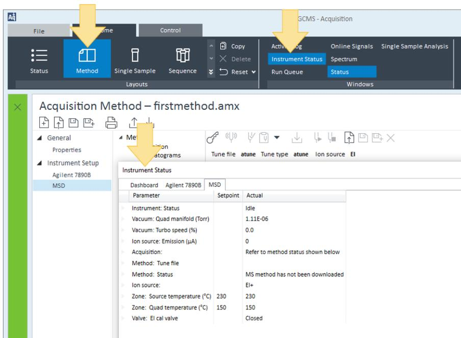
Figure 41. MSD tab Temperatures and Vacuum
