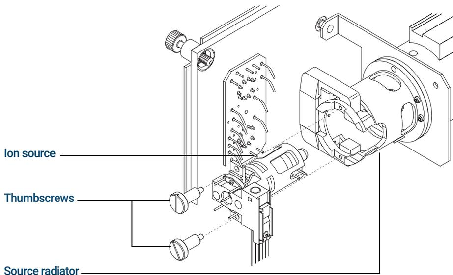
Figure 80. Installing the CI source
