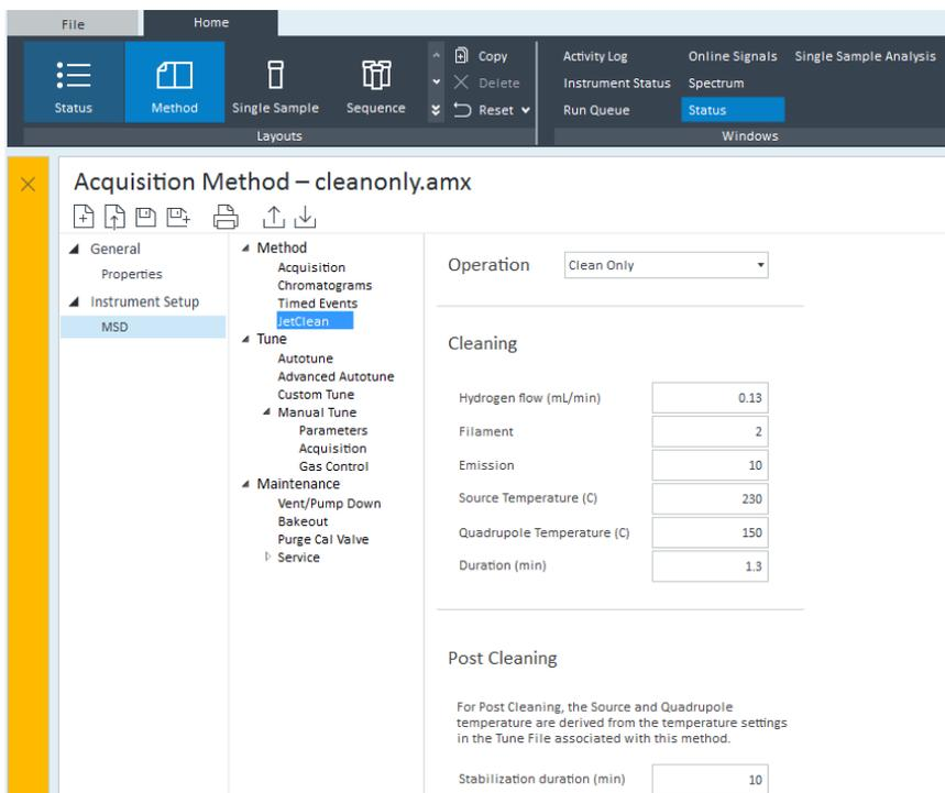
The screenshot displays the software interface for configuring an acquisition method. The title bar reads "Acquisition Method – cleanly.amx". The left sidebar shows a tree view with "MSD" selected under "Instrument Setup". The main panel is divided into three sections:
