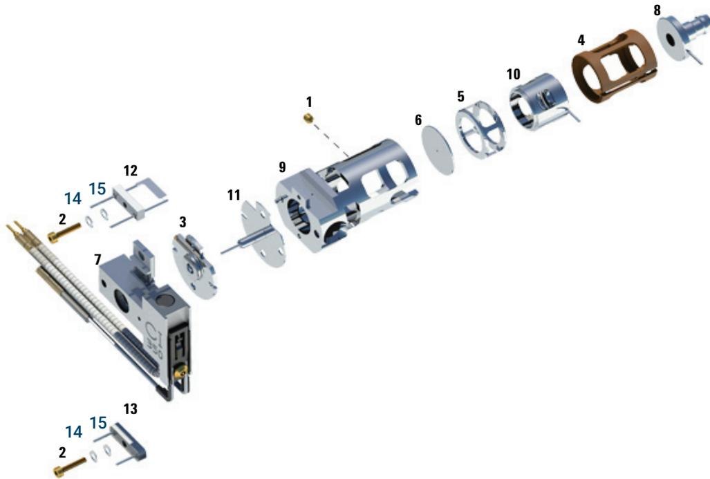
Figure 76. Disassembling the CI source
