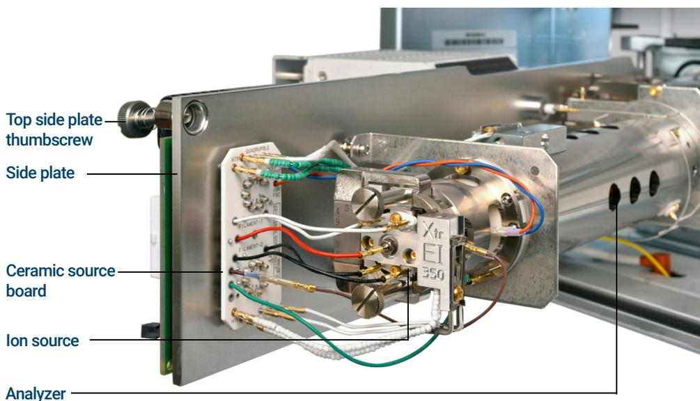
Figure 48. The analyzer chamber for an Inert+ model MSD
