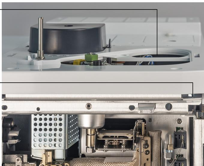
Figure 13. GC inlet cover and compression bolt access plate
