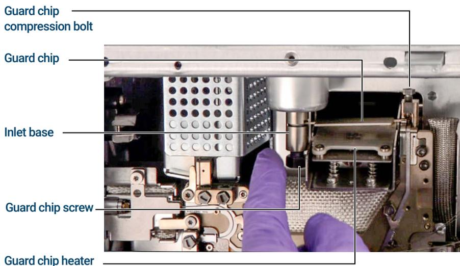
Figure 14. Guard chip and related parts
