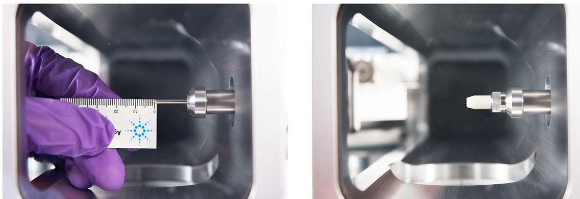
Figure 6. Installing a capillary column in the GC/MSD interface for an EI HES source.
