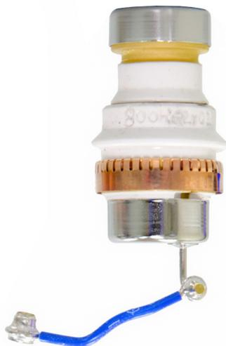
Figure 70. Electron multiplier horn
