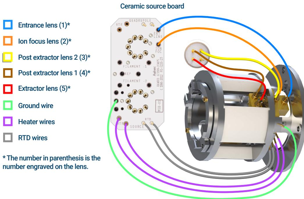
Figure 71 Wiring between the ceramic source board/feedthrough connector and the EI HES radiator
