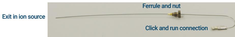
Figure 17. 9000 GC/MS Tail removed from GC/MSD Interface
