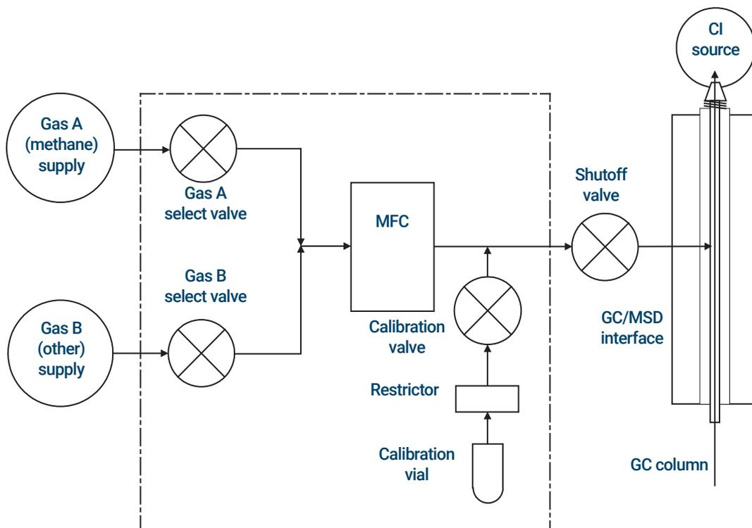
Figure 44. Reagent gas flow control module schematic
