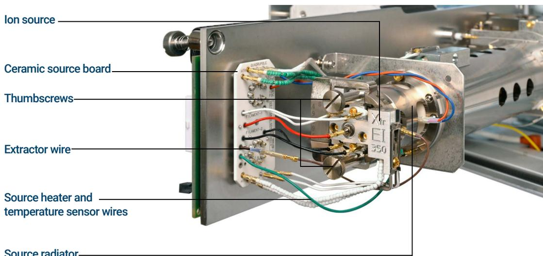
Figure 68. Installing the EI source
