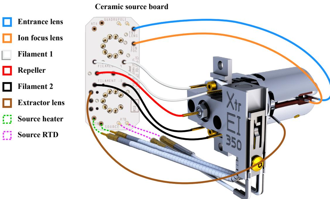
Figure 57 Wiring for the EI XTR Source
