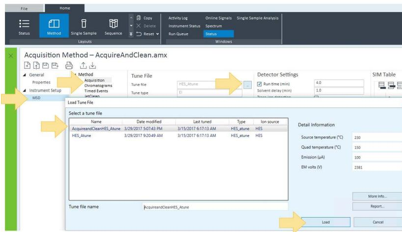
Figure 36. Select a Tune file to Load
