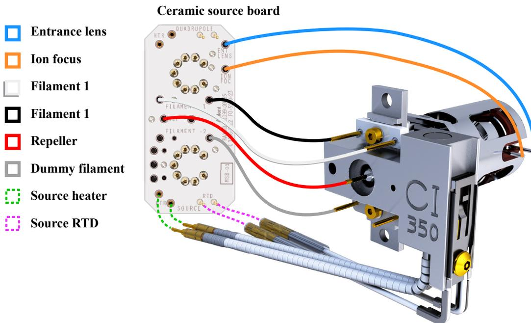
Figure 75 Wiring between the ceramic source board and the source
