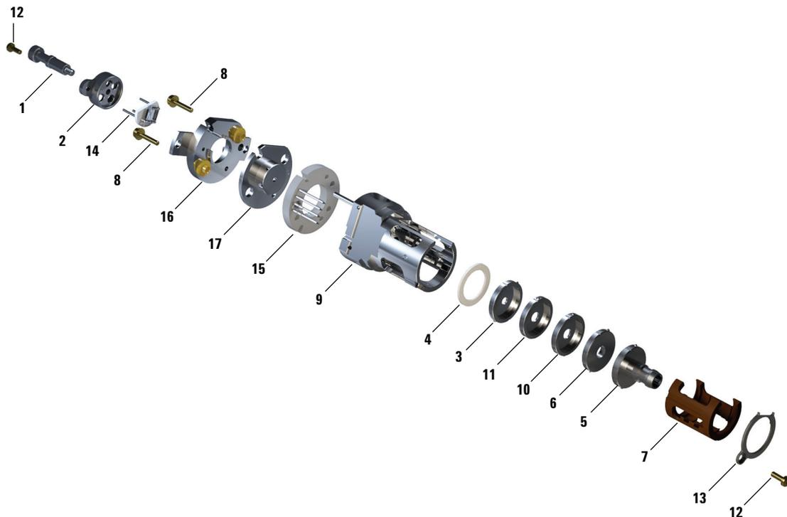
Figure 51 Exploded parts view of the EI HES
