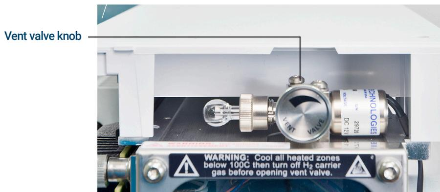
Figure 42 Vent valve knob
