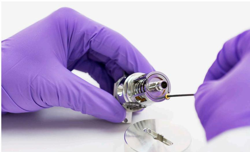
Figure 54 Secure the lens screw and lock ring insulator
