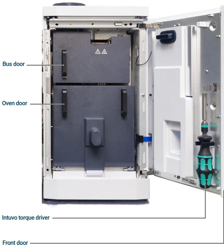
Figure 11. 9000 GC front door, bus door, oven door, and Intuvo torque driver
