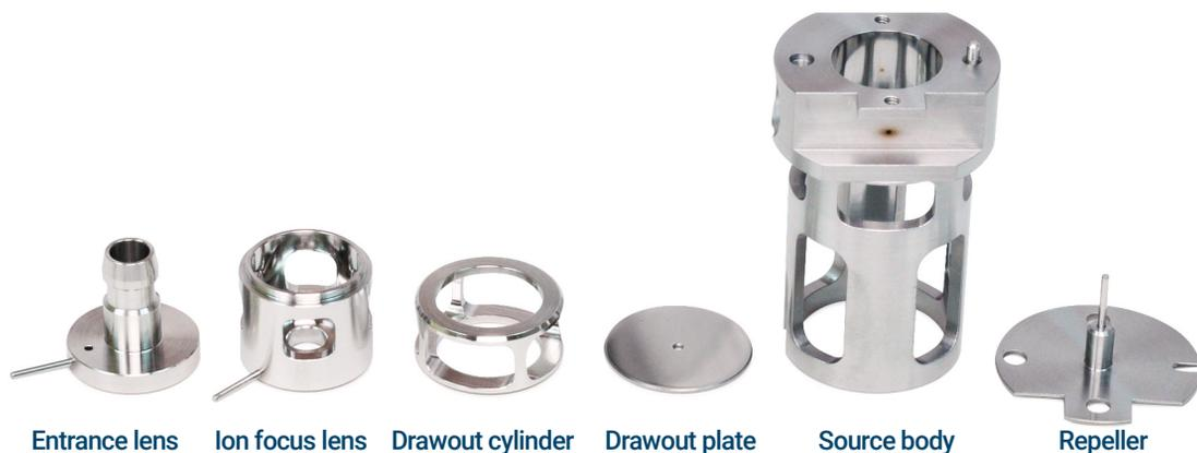
Figure 77. CI source parts to be cleaned
