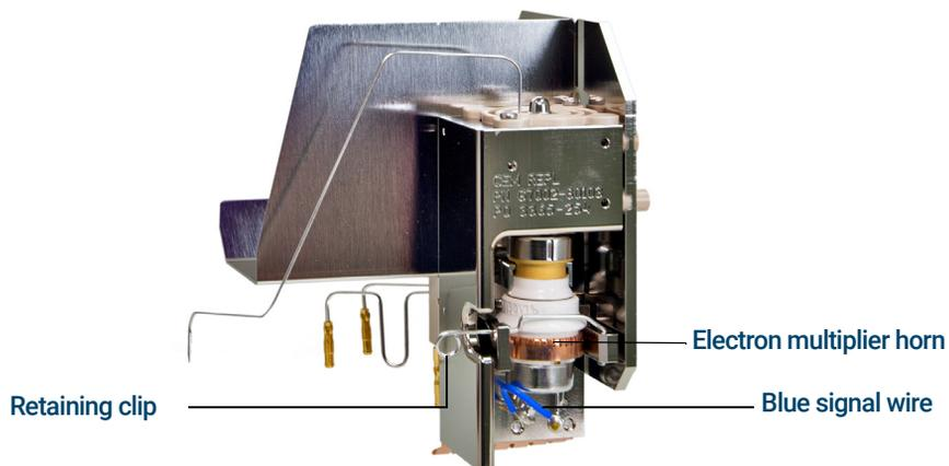
Figure 69. Replacing the EM horn on a Series 2 Detector
