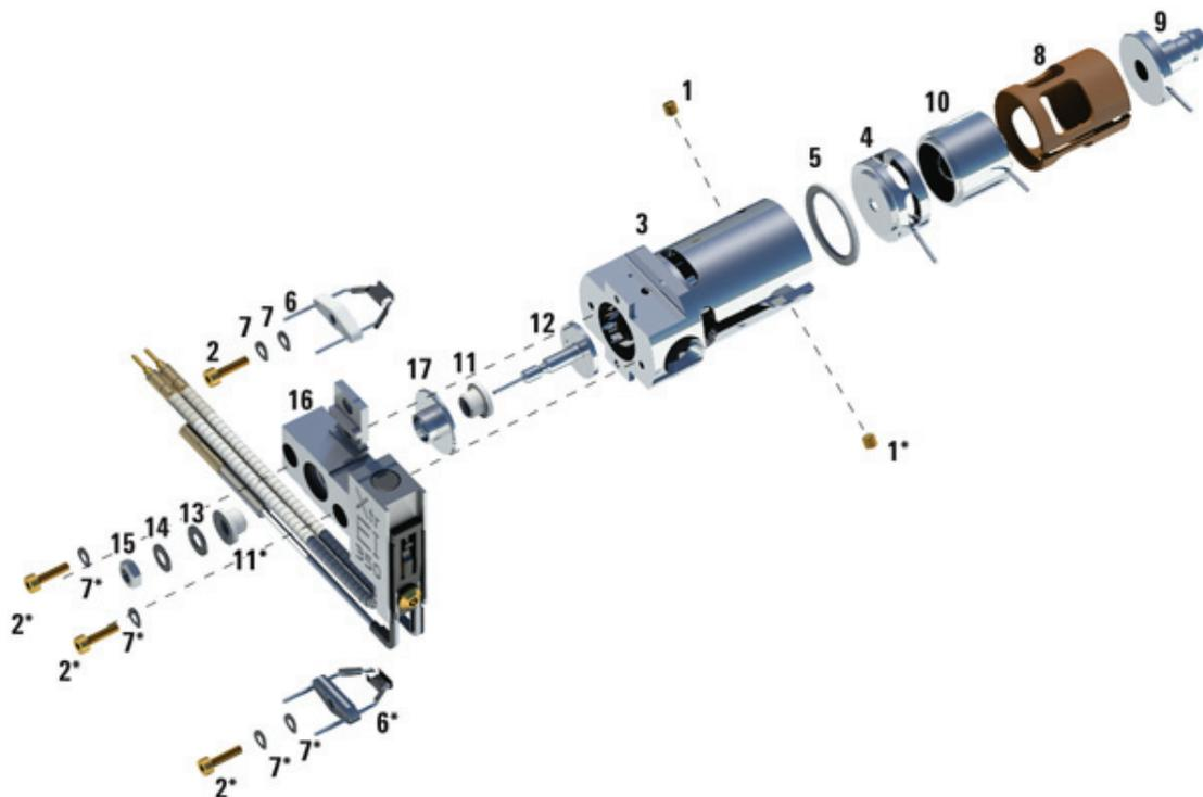
Figure 63. Cleaning the EI HydroInert source
