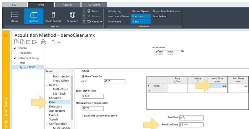
Figure 29. Hold Time and Post Run Time settings
