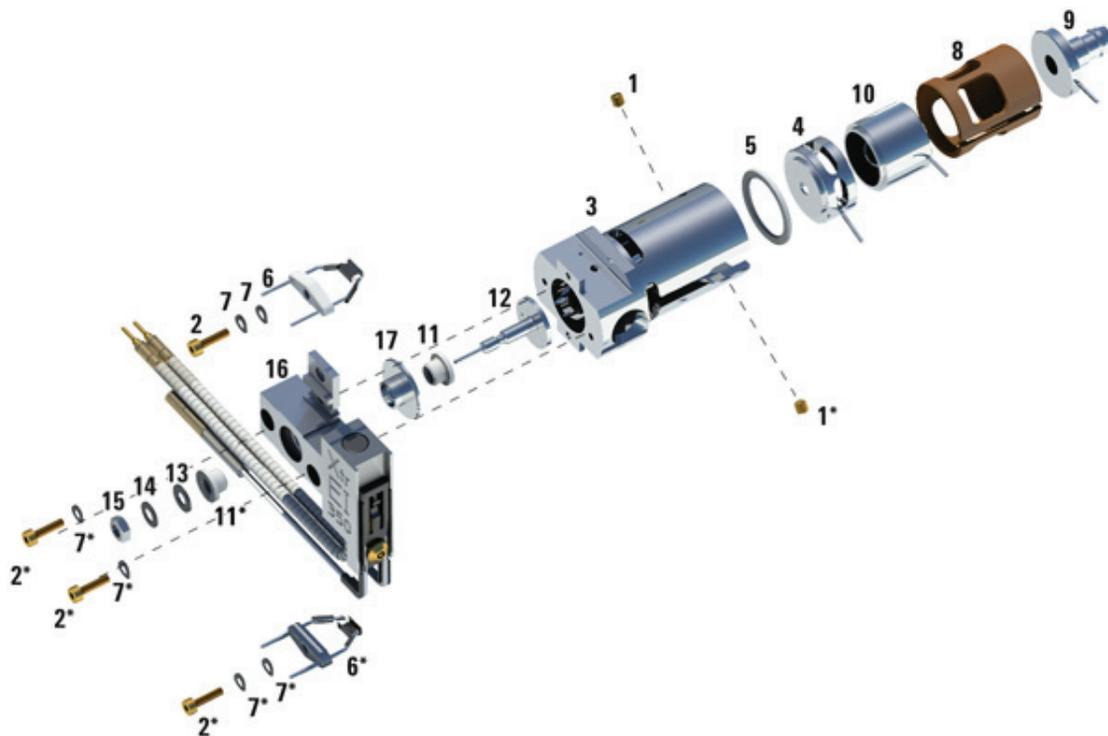
Figure 65. Assembling the EI XTR source
