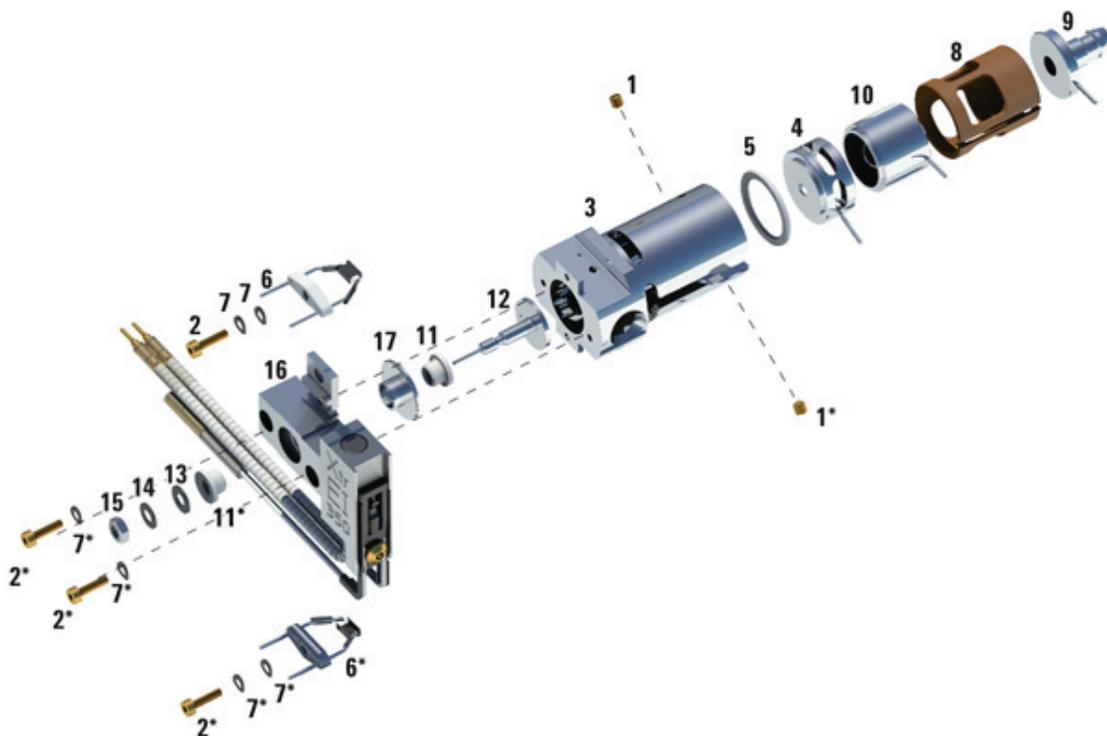
Figure 60. Disassembling the EI XTR source
