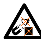
Strong magnetic field. Keep pacemakers and magnetic data storage devices clear from this area.
