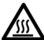
Dangerous surface temperatures
