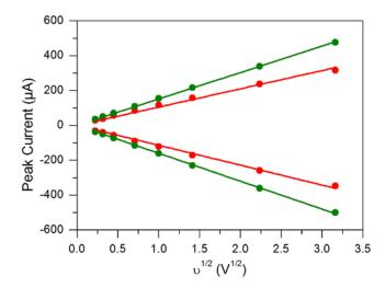
**Figure S4.2:** Plot for the peak current  $i_p$  as a function of the square root of the scan rate  $v^{1/2}$  for the data sets at 50 mM electrolyte concentration, compensated (red) or not (green) for the ohmic drop.
