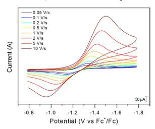
**Figure S5.1**: Voltammograms of the reduction of O<sub>2</sub> in CH<sub>3</sub>CN with 250 mM of [NBu<sub>4</sub>][PF<sub>6</sub>] at various scan rates. Data collected on a 3 mm diameter glassy carbon working electrode, with a platinum counter electrode and a silver wire pseudo-reference electrode in a fritted compartment.
