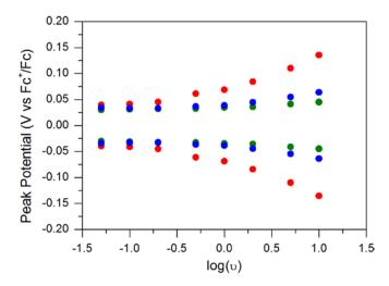
**Figure S3.3**: Plot of the anodic and cathodic peak potentials as a function of the log of scan rate ("trumpet plot") for the three datasets: 50 mM electrolyte concentration uncompensated (red), compensated (green) and 250 mM electrolyte uncompensated (blue).
