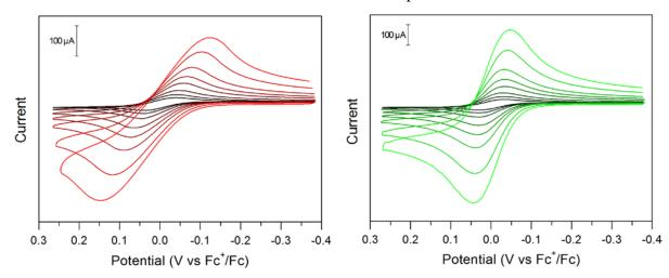
Figure S3.1: Cyclic voltammograms at 0.05, 0.1, 0.2, 0.5, 1, 2, 5 and 10 V/s of a 1 mM ferrocene solution in CH<sub>3</sub>CN with 50 mM of [NBu<sub>4</sub>][PF<sub>6</sub>] as supporting electrolyte. The data was collected without (red, left) and with (green, right) ohmic drop compensation. Data collected on a 3 mm diameter glassy carbon working electrode, with a platinum counter electrode and a silver wire pseudo-reference electrode in a fritted compartment.
