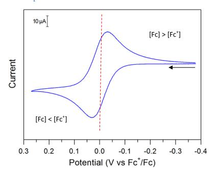
**Figure S1.1.** Voltammogram of a ferrocene solution, referenced to ferrocene. The dashed red line indicates  $E_{1/2}$ .
