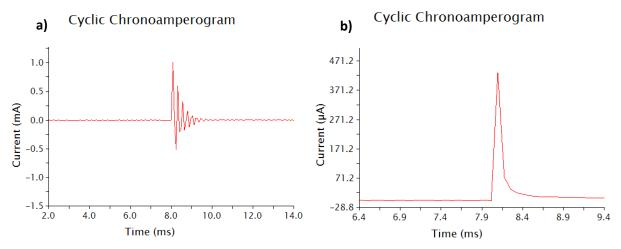
**Figure 2.2.** Cyclic (or double potential step) chronoamperograms that demonstrate a) oscillations and b) no oscillations.
