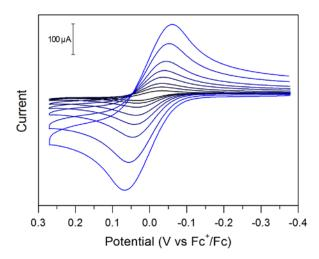
**Figure S3.2**: Cyclic voltammograms at 0.05, 0.1, 0.2, 0.5, 1, 2, 5 and 10 V/s of a 1 mM ferrocene solution in CH<sub>3</sub>CN with 250 mM of [NBu<sub>4</sub>][PF<sub>6</sub>] as supporting electrolyte. No ohmic drop compensation was used. Data collected on a 3 mm diameter glassy carbon working electrode, with a platinum counter electrode and a silver wire pseudo-reference electrode in a fritted compartment.
