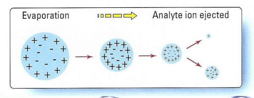
Figure 5. Desorption of ions from solution
