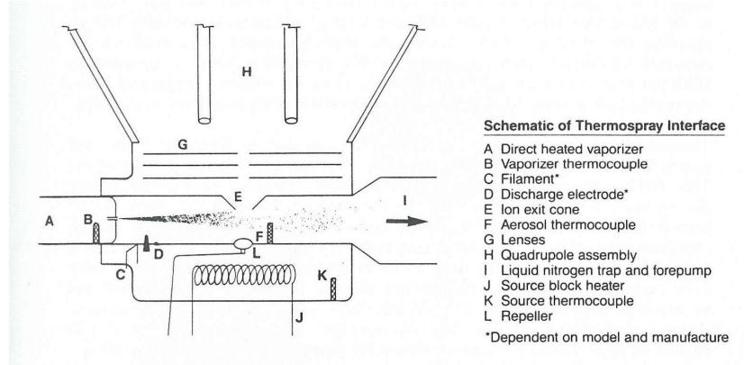
**Figure 4.** Schematic of a thermospray LC/MS interface. [From reference 11]
