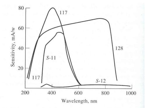
**Figure 7-28** Spectral response of some typical photoemissive surfaces. *(From F. E. Lytle, Anal. Chem., 1974, 46, 546A. Copyright 1974 American Chemical Society.)*
