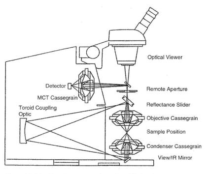
**Figure 4.24** IR microscope schematic with the detector integrated into the microscope. The microscope is usually coupled to a light port on the side of the FTIR spectrometer. The FTIR spectrometer supplies a modulated, collimated beam of light to the microscope. Courtesy of PerkinElmer Instruments, Shelton, CT (www.perkinelmer.com). (From Coates, used with permission.)
