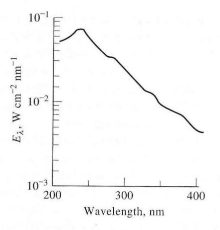
Figure 13-11 Output from a deuterium lamp.
