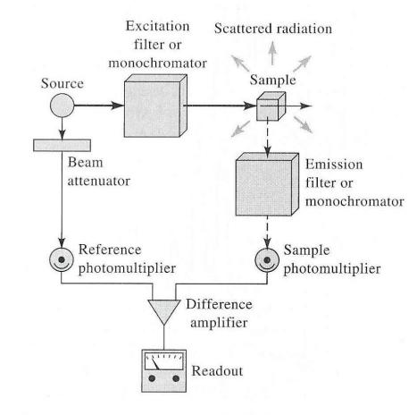
**Figure 15-4** Components of a fluorometer or a spectro-fluorometer.
