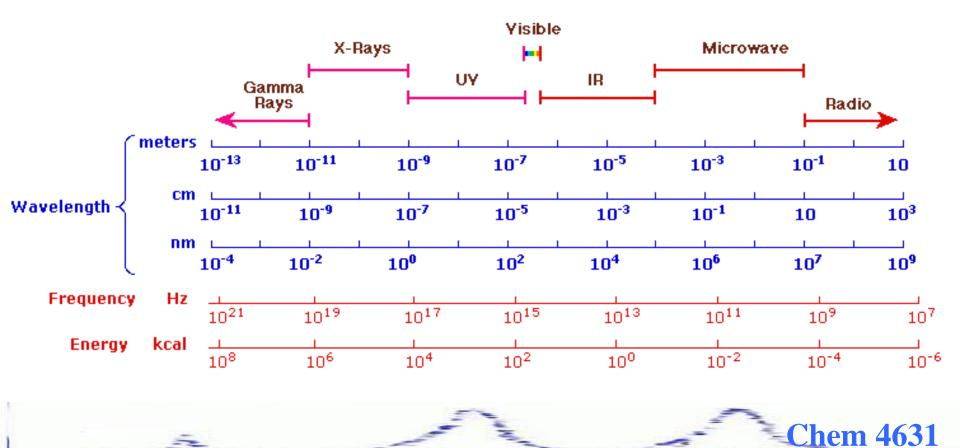
**Components of Optical** Instruments **UV, Fluorescence to IR Optical spectroscopy is based on:** – absorption - fluorescence - phosphorescence - scattering - emission - chemiluminescence
