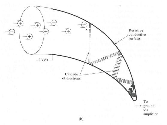
**Figure 11-2** (a) Discrete dynode electron multiplier. Dynodes are kept at successively higher potentials via a multistage voltage divider. (b) Continuous dynode electron multiplier. (*Adapted from J. T. Watson,* Introduction to Mass Spectrometry, *p. 247. New York: Raven Press, 1985. With permission.*)
