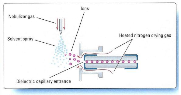
Figure 4. Electrospray ion source
