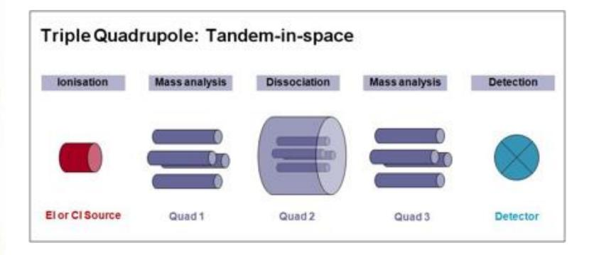
Three Quadrupoles (Quad 1, Quad 2, and Quad 3) are lined up in a row. Precursor ions are selected in Quad 1 and sent to Quad 2 for dissociation (fragmentation). The generated product ions are sent to Quad 3 for mass scanning.
