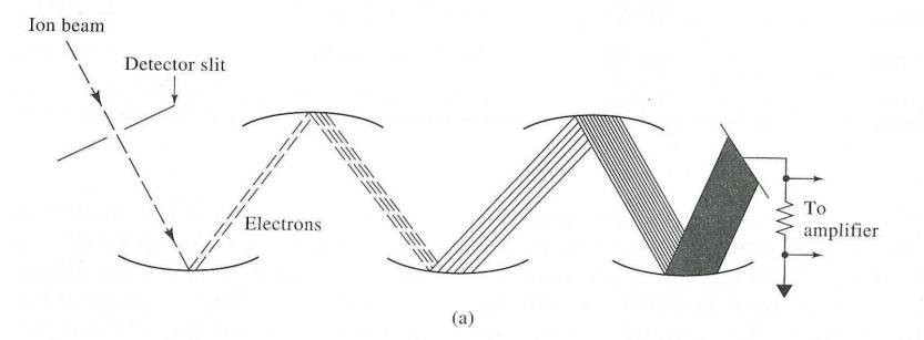
**Figure 11-2** (a) Discrete dynode electron multiplier. Dynodes are kept at successively higher potentials via a multistage voltage divider. (b) Continuous dynode electron multiplier. (*Adapted from J. T. Watson,* Introduction to Mass Spectrometry, *p. 247. New York: Raven Press, 1985. With permission.*)
