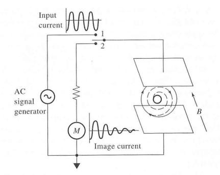
**Figure 20-16** Path of an ion in a strong magnetic field. Inner solid line represents the original circular path of the ion. Dashed line shows spiral path when switch is moved briefly to position 1. Outer solid line is new circular path when switch is again opened.
