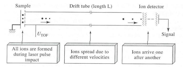
**Figure 11-8** Principle of a time-of-flight mass spectrometer. A bunch of ions produced by a laser probe is accelerated into the drift tube where separation occurs. (From A. H. Verbueken, F. J. Bruynseels, R. Van Grieken, and F. Adams, in Inorganic Mass Spectrometry, p. 186. F. Adams, R. Gijbels, and R. Van Grieken, Eds. New York: Wiley, 1988. With permission.)
