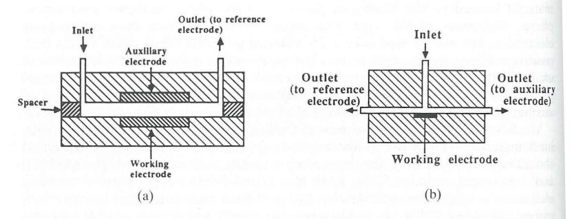
Fig. 5.27. Schematic illustration of (a) thin-layer and (b) wall-jet amperometric flow-cells.
