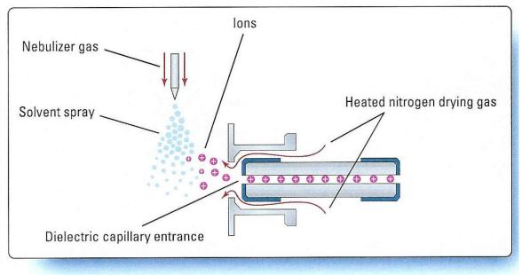
Figure 4. Electrospray ion source
