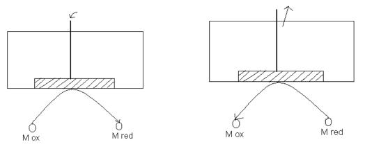
The electrochemical reaction occurs at the interface between the w.e. and solution. One major problem - reaction products can accumulate and adhere to electrode surface (fouling, poisoning) eventually passivating the surface. Electrode must be removed and polished or cleaned by potential pulsing.
