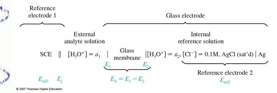
Indicator Electrodes Membrane Electrodes pH Electrode -- glass electrode
