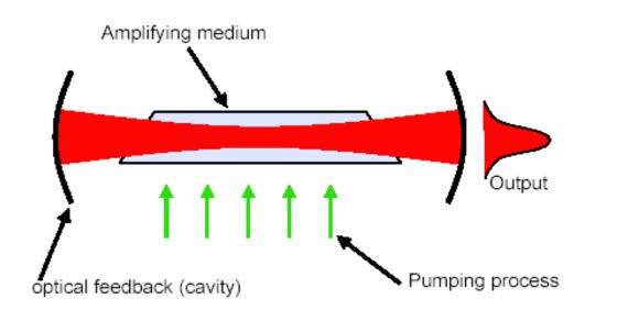
Once the cascade begins the laser functions as a resonator, passing the radiation back and forth through the medium using mirrors. This generates even more photons – "amplification".
