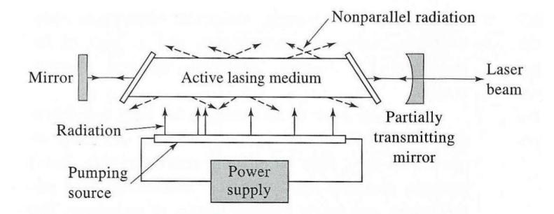
Once the cascade begins the laser functions as a resonator, passing the radiation back and forth through the medium using mirrors. This generates even more photons – "amplification".
