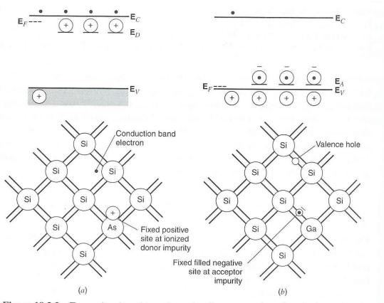
**Figure 18.2.3** Energy bands and two-dimensional representation of extrinsic semiconductor lattices. (*a*) *n*-type. (*b*) *p*-type.
