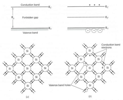
**Figure 18.2.2** Energy bands and two-dimensional representation of an intrinsic semiconductor lattice. (*a*) At absolute zero (or  $\mathbf{E}_{g} >> \&T$ ), assuming a perfect lattice; no holes or electrons exist. (*b*) At a temperature where some lattice bonds are broken, yielding electrons in the conduction band and holes in the valence band.  $\mathbf{E}_{F}$  represents the Fermi level in this intrinsic semiconductor.
