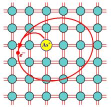
Fig. 5.9: Arsenic doped Si crystal. The four valence electrons of As allow it to bond just like Si but the fifth electron is left orbiting the As site. The energy required to release to free fifth-electron into the CB is very small.
