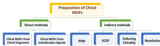
Scheme 1. The synthetic strategies for the preparation of chiral MOFs by direct and indirect methods.
